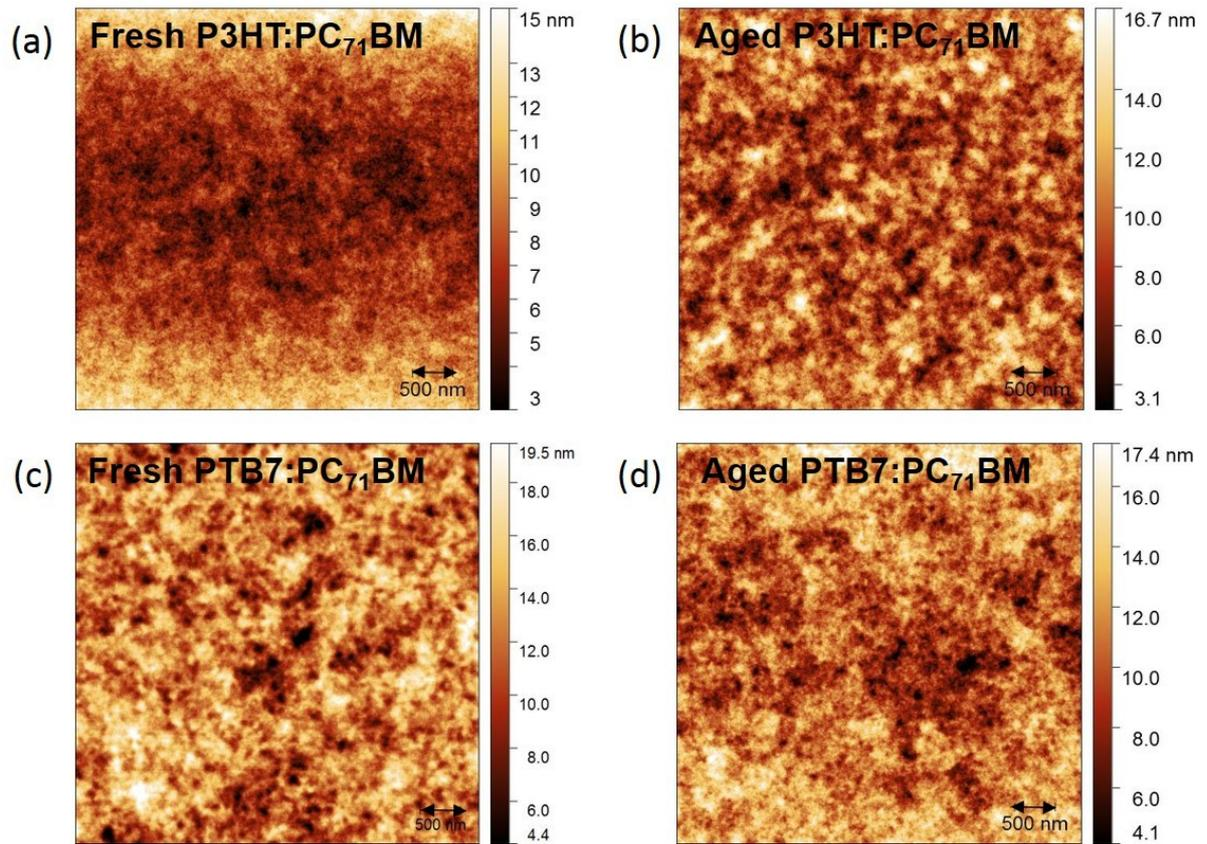
FIG. S7. AFM images (5  $\mu\text{m} \times 5 \mu\text{m}$ ) of P3HT:PC<sub>71</sub>BM and PTB7:PC<sub>71</sub>BM films under both fresh and aged conditions. The RMS surface roughness extracted from AFM images are summarized in the following table:
