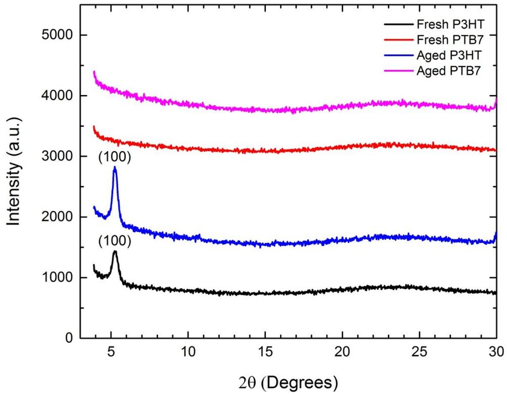
FIG. S8. X-ray diffraction patterns of P3HT:PC<sub>71</sub>BM and PTB7:PC<sub>71</sub>BM films under both fresh and aged conditions
