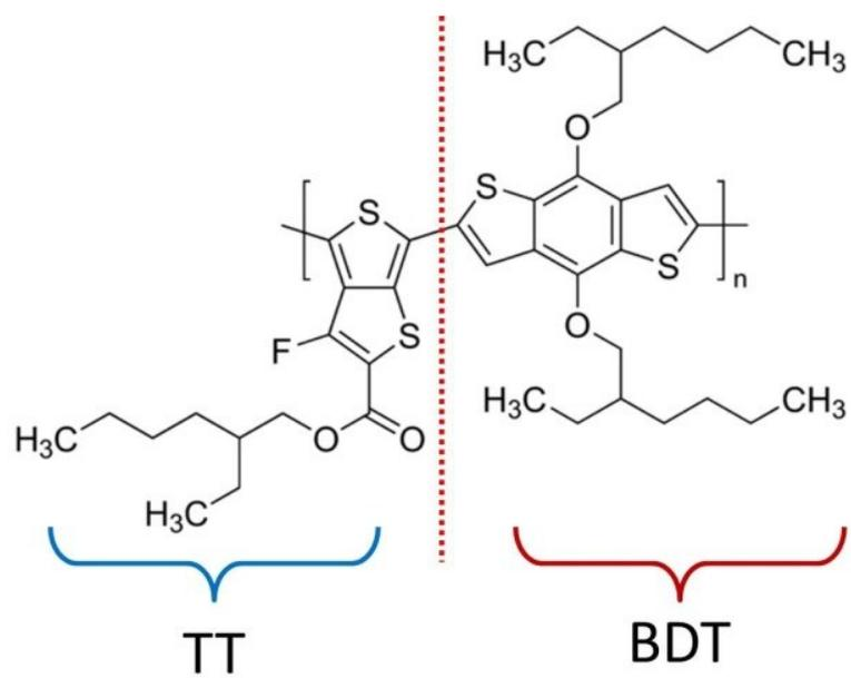
FIG. S9. Chemical structures of the repeat unit consisting BDT and TT for the polymer donor PTB7
