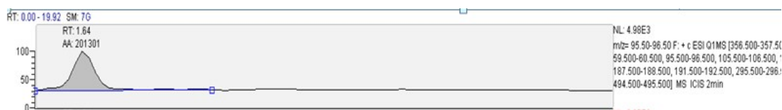
Fig. S17. The LC-MSMS scan of byproducts formed during the chlorination of FF with the mass/ionization ( m/z ) values of 96
