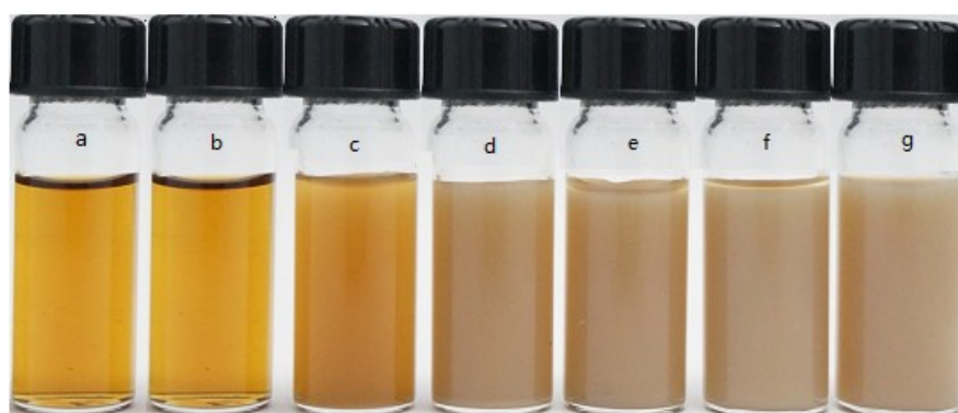
Fig. s1 The optical photographs (under) of His-GQD system after added 0.0 (a), 0.01 (b), 0.02 (c), 0.03 (d), 0.04 (d), 0.05 (e), 0.06 (f) and 0.07 (g) of \text{Zn}^{2+}
