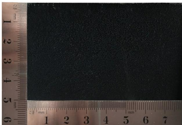
**Fig. S4** The optical image of the Cu/ZnO heterostructured film grown on large area of Zn substrate (40 cm<sup>2</sup>).
