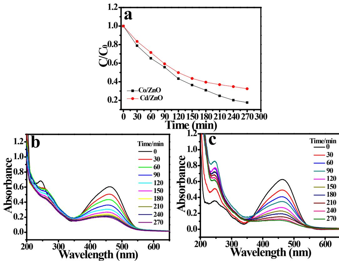
**Fig. S7** (a) Photocatalytic degradation and (b, c) time-dependent UV-vis absorption spectra of MO solution with different catalysts: (b) Cd/ZnO and (c) Co/ZnO heterostructured films.
