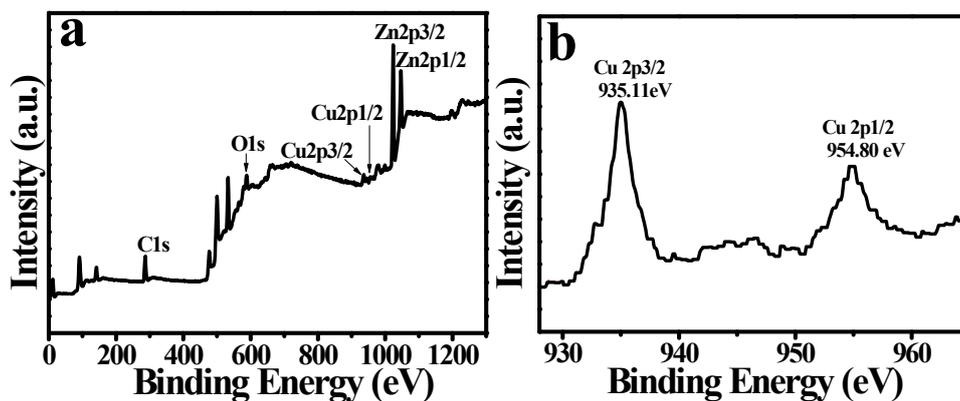
**Fig. S9** XPS spectra of the pine tree-like Cu/ZnO heterostructured film on zinc substrate after the fifth catalysis cycles: (a) survey spectrum, and core-level spectra of (b) Cu 2p
