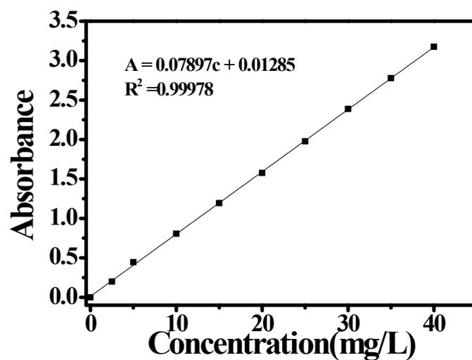
**Fig. S5** The linear calibration curve for a series of standard MO aqueous solutions (0 mg/L, 2.5 mg/L, 5 mg/L, 10 mg/L, 15 mg/L, 20 mg/L, 25 mg/L, 30 mg/L, 35 mg/L and 40 mg/L).
