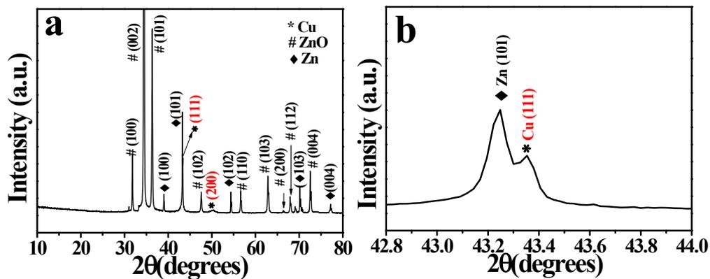
**Fig. S8** (a) The XRD pattern of pine tree-like Cu/ZnO heterostructured film on zinc substrate after the fifth catalysis cycles. (b) Fine-scanned Zn(101) and Cu(111) peaks of the Fig.S8 a.
