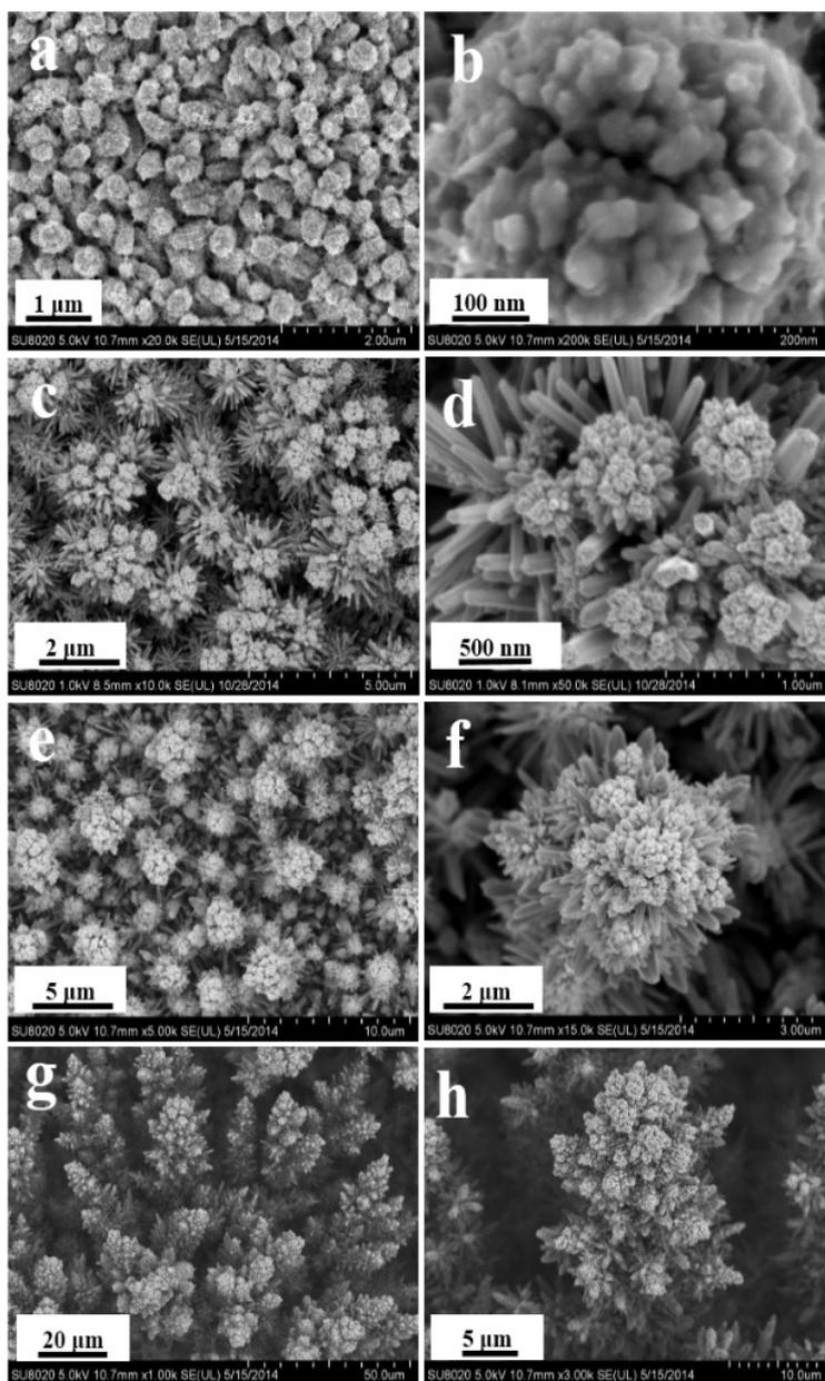
**Figure S1.** FESEM images of the as-obtained Cu/ZnO heterostructured film on zinc substrate at different reaction times: (a-b) 1 h, (c-d) 3 h, (e-f) 6 h, (g-h) 12 h.
