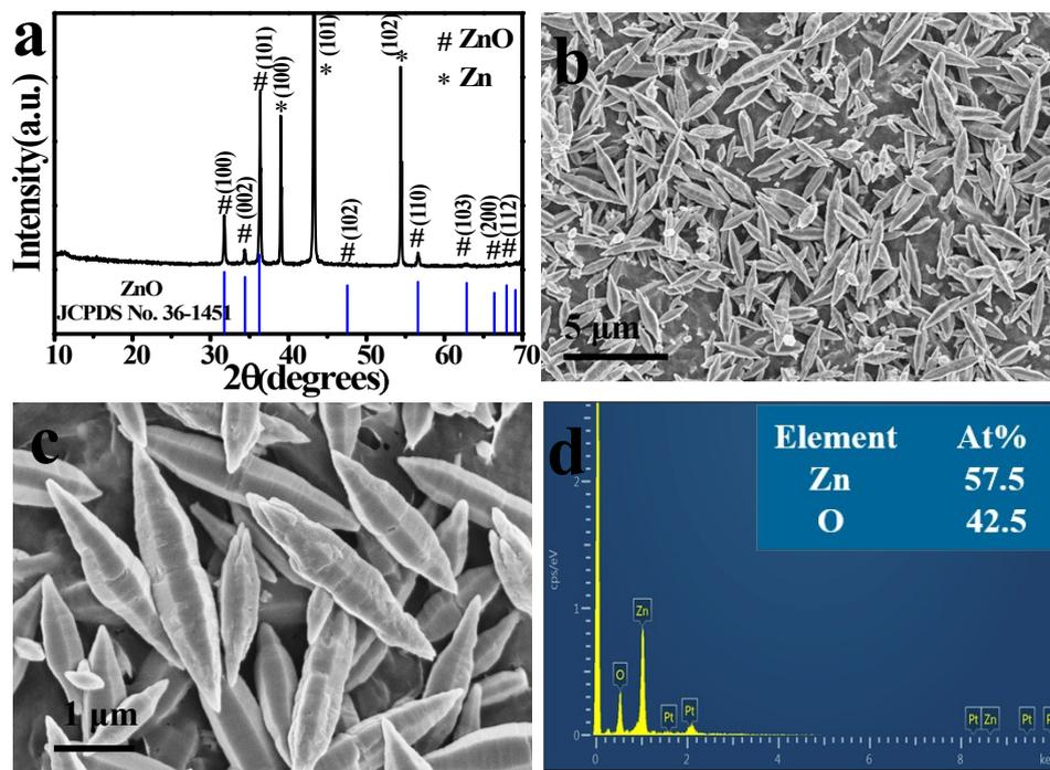
Fig. S3 (a) XRD pattern, (b, c) FESEM images and (d) EDS spectrum of the ZnO nanospindle films grown on zinc substrate.
