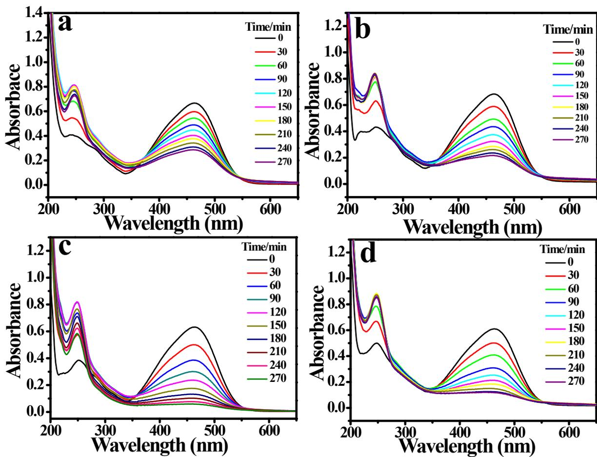
Fig. S6 Time-dependent UV-vis absorption spectra of MO aqueous solution under visible light irradiation in the presence of different photocatalysts: (a) ZnO, and Cu/ZnO heterostructures prepared with different concentrations of  $\text{Cu}^{2+}$ : (b) 0.2 mM (S1), (c) 0.6 mM (S2) and (d) 2.0 mM (S3).
