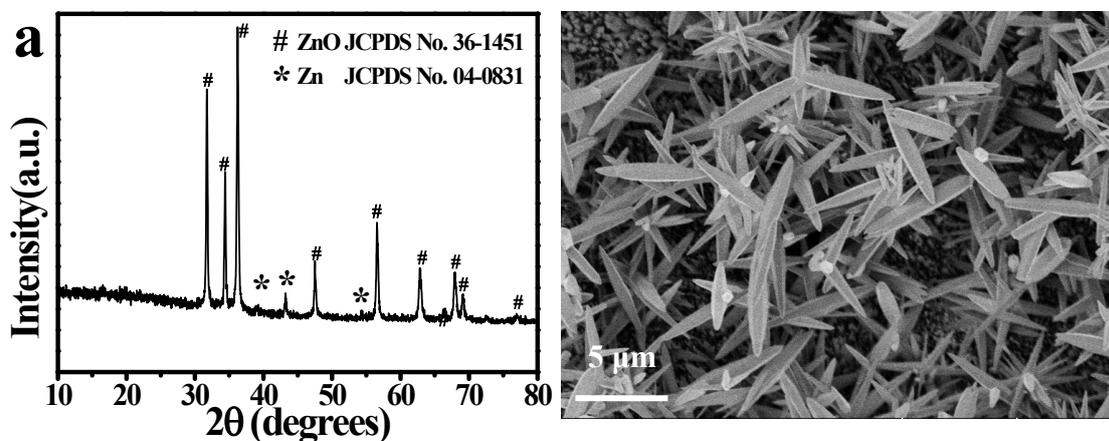
**Fig. S11** (a) XRD pattern and (b) FESEM image of the bare ZnO nanospindle film on Zn substrate.
