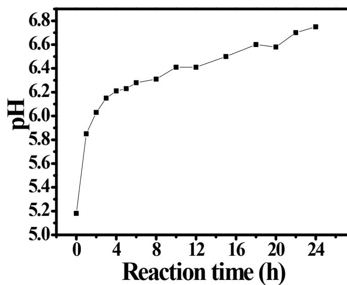
**Fig. S2** The pH values of the reaction media as a function of reaction time during the synthesis of Cu/ZnO heterostructured films ( $c_{\text{Cu}^{2+}} = 0.6 \text{ mM}$ ).
