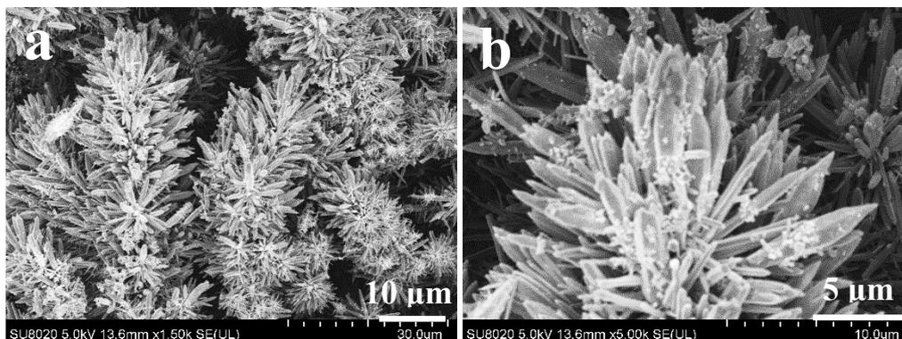
Fig. S10 (a) Low and high resolution FESEM images of pine tree-like Cu/ZnO heterostructured film on zinc substrate after the fifth catalysis cycles
