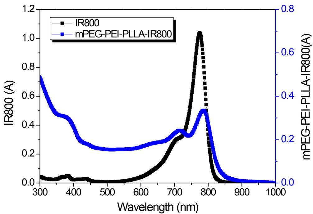
**Figure S10.** UV-Vis spectrum of IR800 NIR dye before and after conjugation to the particles.
