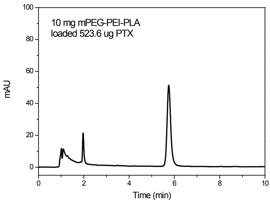
**Figure S4.** HPLC chromatograph of mPEG-PEI-PLLA-PTX PBS solution, with PTX appearing at 5.7 min.
