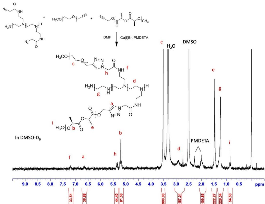
**Figure S3.**  $^1\text{H}$  NMR spectrum of mPEG-PEI-PLLA (300 MHz, DMSO- $\text{D}_6$ ).
