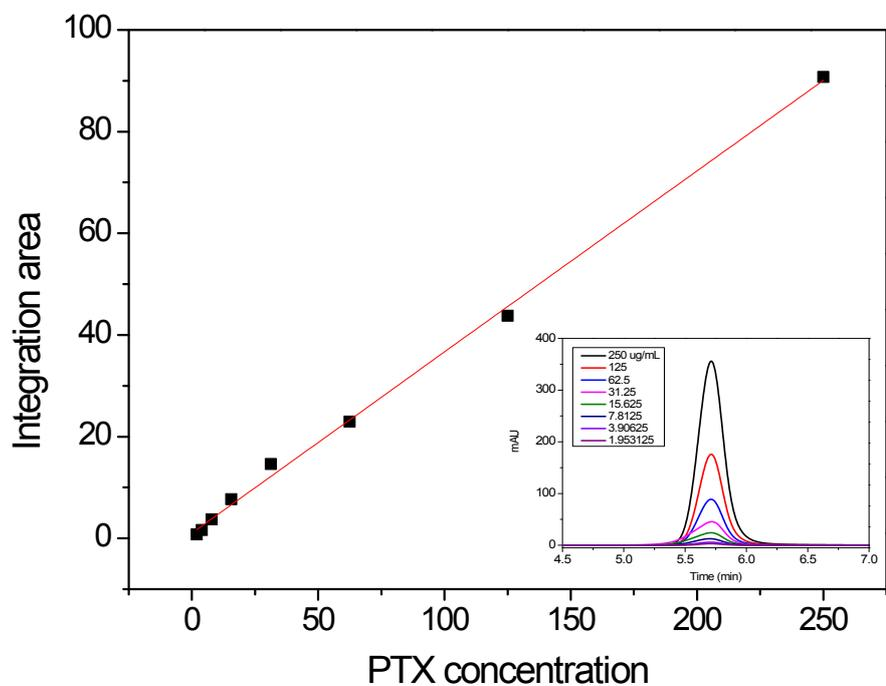
**Figure S6.**PTX calibration curve. The 228nm peak area at 5.7 min was utilized to calculate integration area.
