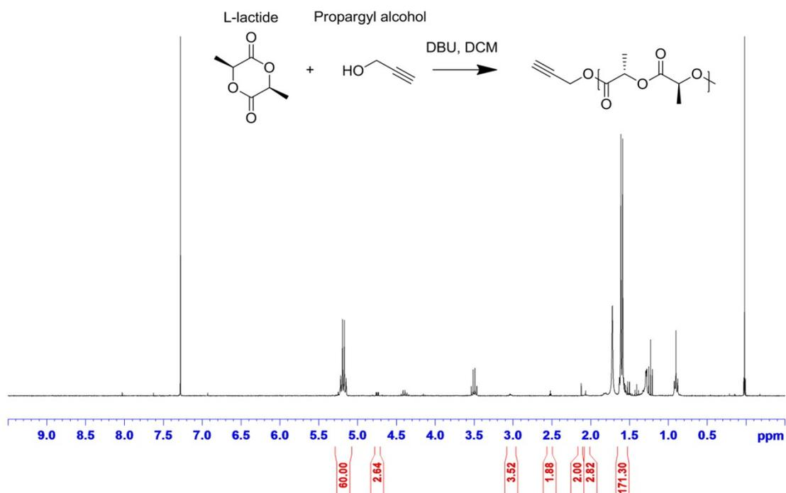
Figure S2. <sup>1</sup>H NMR spectrum of PLLA-alkyne (300 MHz, CDCl<sub>3</sub>).
