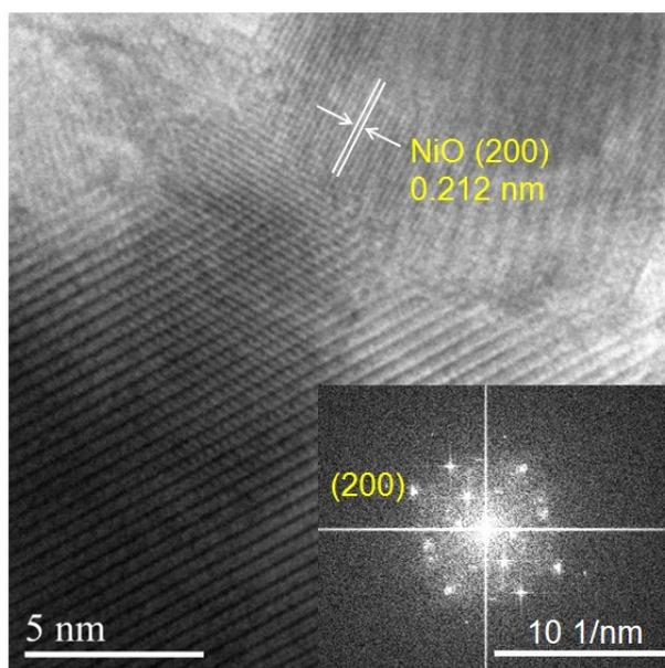
**Figure S3** HRTEM lattice image and corresponding fast Fourier transform (FFT) pattern (inset) of Co<sub>2</sub>NiAlO-800.
