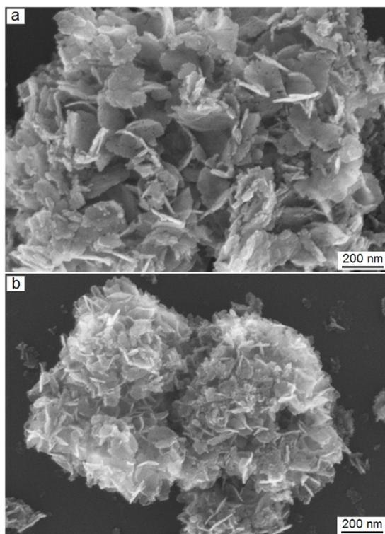
**Figure S4** SEM images of the used catalysts Co<sub>3</sub>AlO-500-u (a) and Co<sub>2</sub>NiAlO-500-u (b) after the stability tests.
