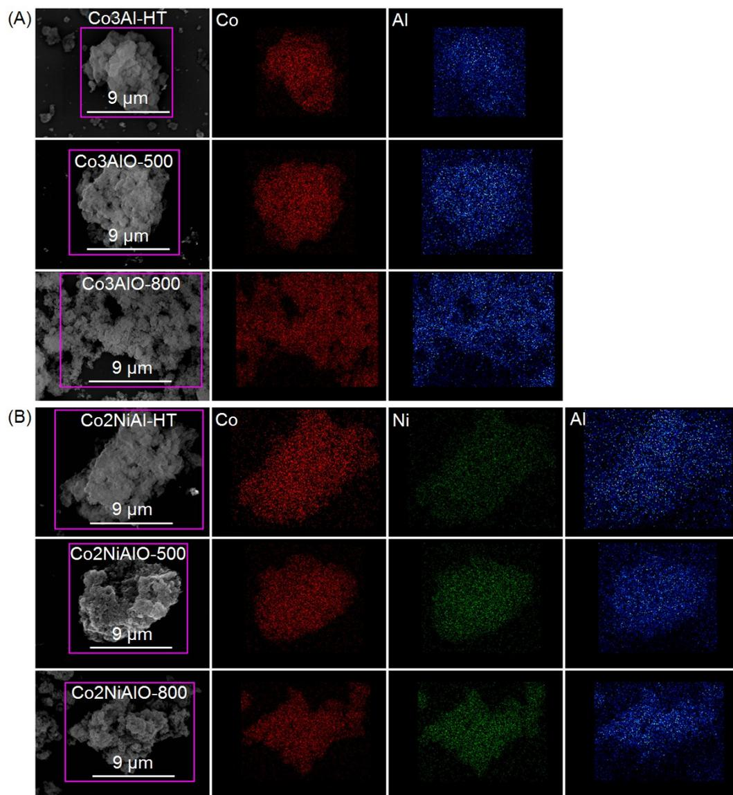
**Figure S2** Mapping of (A) the hydrotalcite precursor Co<sub>3</sub>Al-HT and the catalysts Co<sub>3</sub>AlO-500 and Co<sub>3</sub>AlO-800 and (B) the precursor Co<sub>2</sub>NiAl-HT and the catalysts Co<sub>2</sub>NiAlO-500 and Co<sub>2</sub>NiAlO-800.
