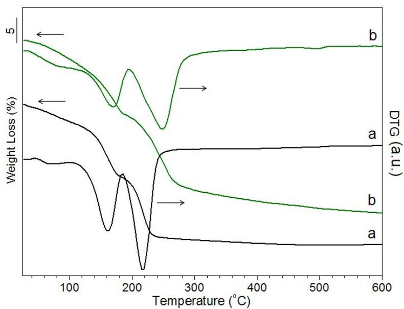
**Figure S1** TG/DTG profiles of the hydroxalcite precursors Co<sub>3</sub>Al-HT (a) and Co<sub>2</sub>NiAl-HT (b).
