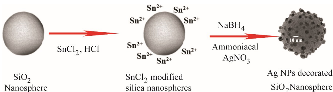
Fig. S2 Schematic illustrations for the decoration of SiO 2 NSs with Ag NPs by modifying the silica surface with Sn 2+ .
