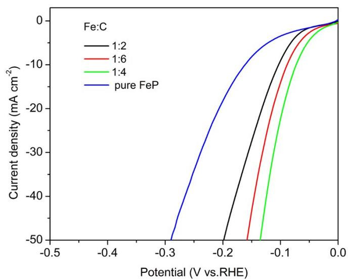
Fig. S4 Polarization curves of FeP/C NCs catalysts synthesized with various Fe/C mole ratio.
