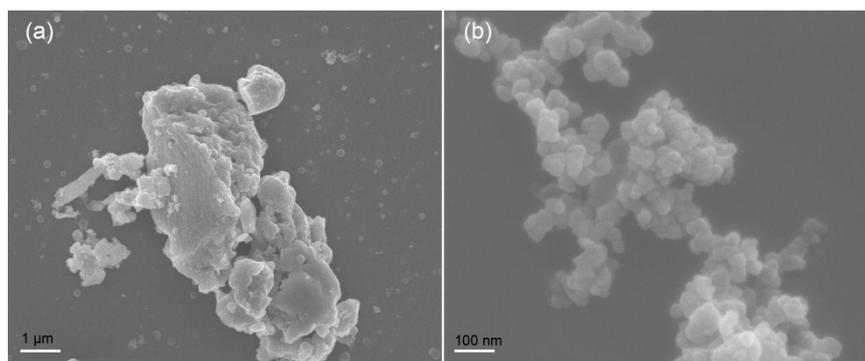
Fig. S1 SEM image of pure FeP (a) and bare carbon black (b).
