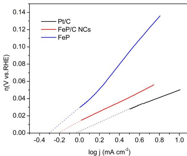
Fig. S6 Calculation of exchange current density for FeP/C NCs, pure FeP and Pt/C.
