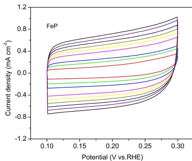
Fig. S7 Cyclic voltammograms (CV) recorded for pure FeP at various scan rates.
