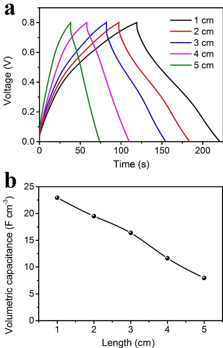
**Figure S11.** Electrochemical performance of fiber-shaped supercapacitors using GrPI@AT yarns of different lengths. **(a)** Voltage profile. **(b)** Volumetric capacitance corresponding to different lengths of GrPI@AT yarns. Current density of  $90 \text{ mA cm}^{-2}$  is used for all cases.
