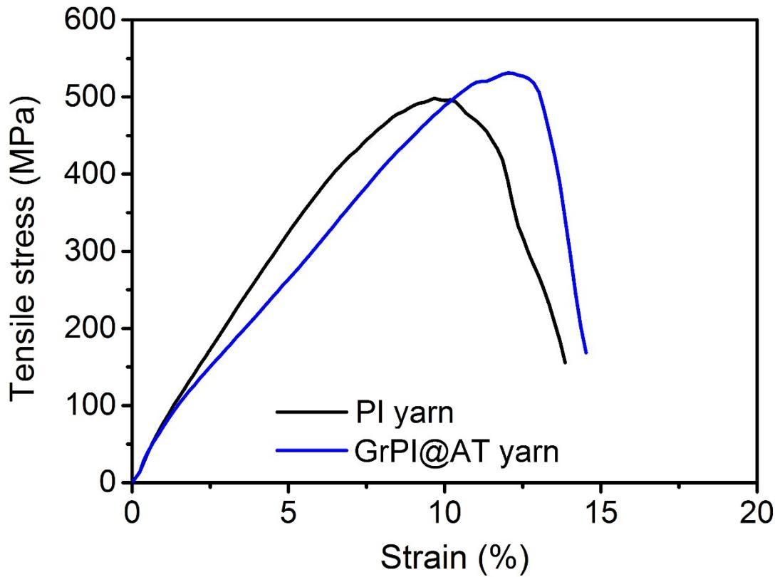
**Figure S10.** Tensile properties of commercial PI yarn and GrPI@AT yarn.
