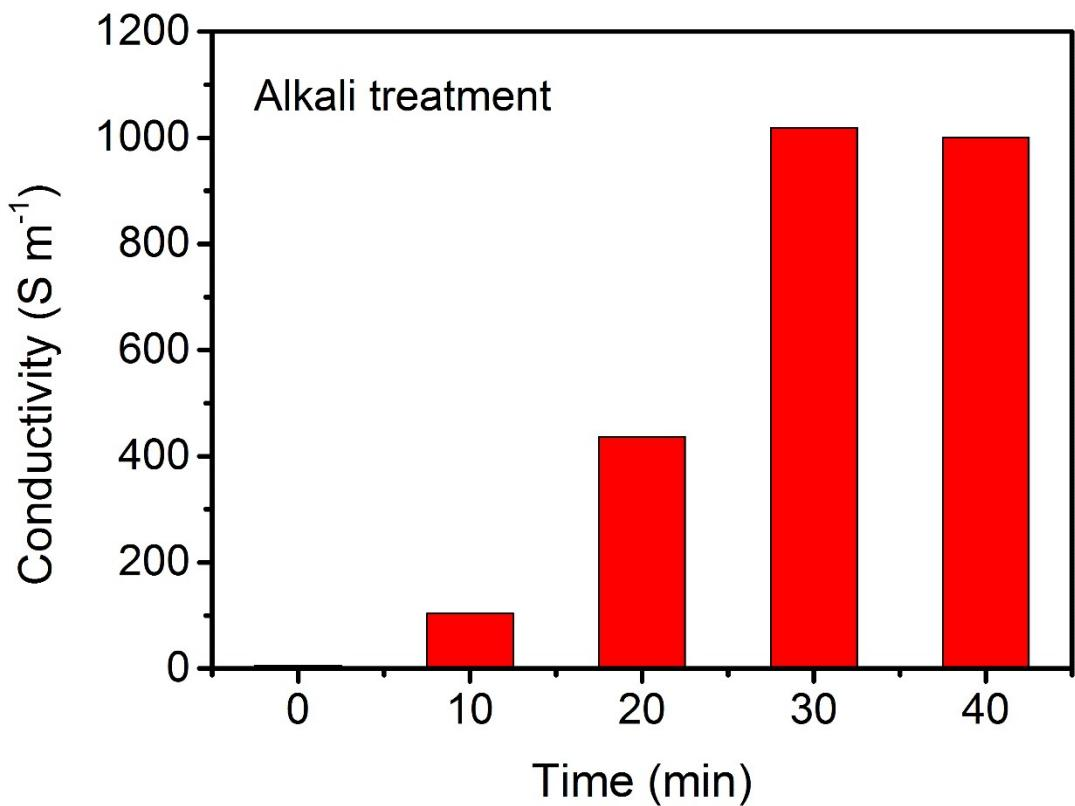
**Figure S7.** Effect of the conductivity of GrPI@AT yarns on the time of alkali treatment.
