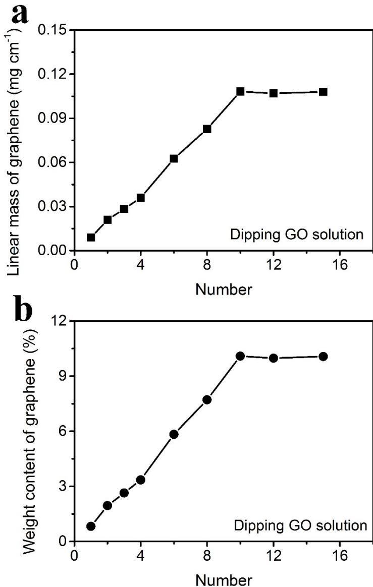
**Figure S6.** (a) Linear mass of graphene on GrPI@AT yarns with increasing the number of dipping GO solution. (b) Weight content of graphene in GrPI@AT yarns with increasing the number of dipping GO solution.
