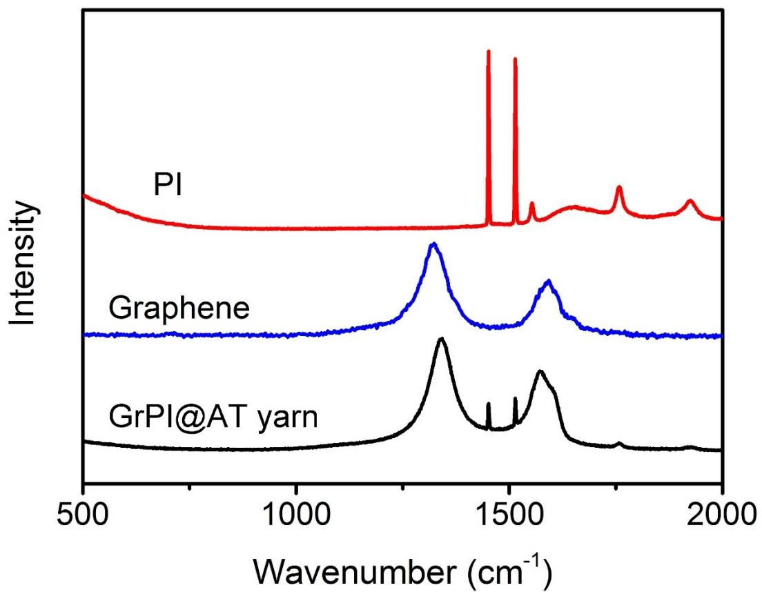
**Figure S4.** Raman spectra of PI yarn, graphene film and GrPI@AT yarn.
