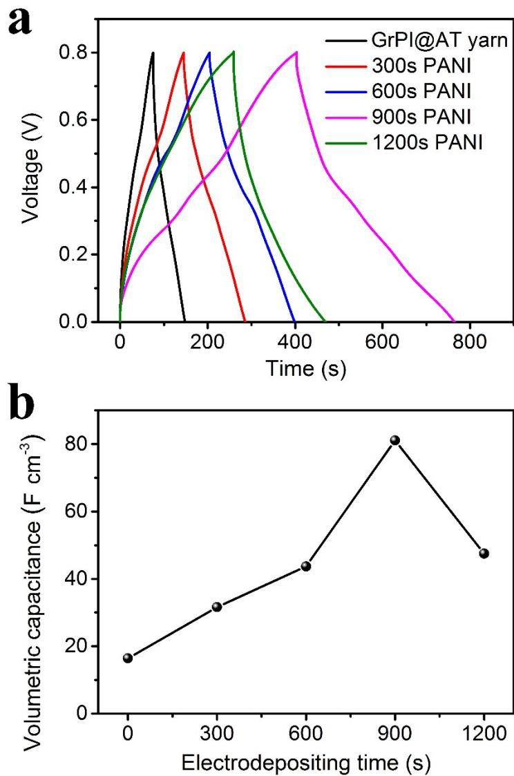
**Figure S12.** Electrochemical performance of fiber-shaped supercapacitors using GrPI@AT-PANI yarns. **(a)** Voltage profile. **(b)** Volumetric capacitance corresponding to different electrodepositing time of PANI. Length of 3 cm and current density of  $90 \text{ mA cm}^{-2}$  are used for all cases.
