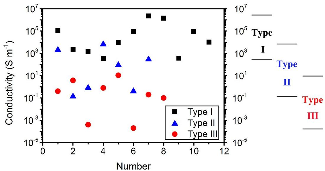
**Figure S1.** Comparison on conductivity of CNT-based or graphene-based fibers (Type I), polymer-matrix composite fibers with CNT or/and graphene coatings (Type II), and polymer-matrix composite fibers with CNT or/and graphene fillers (Type III) (data extracted from Table S1).
