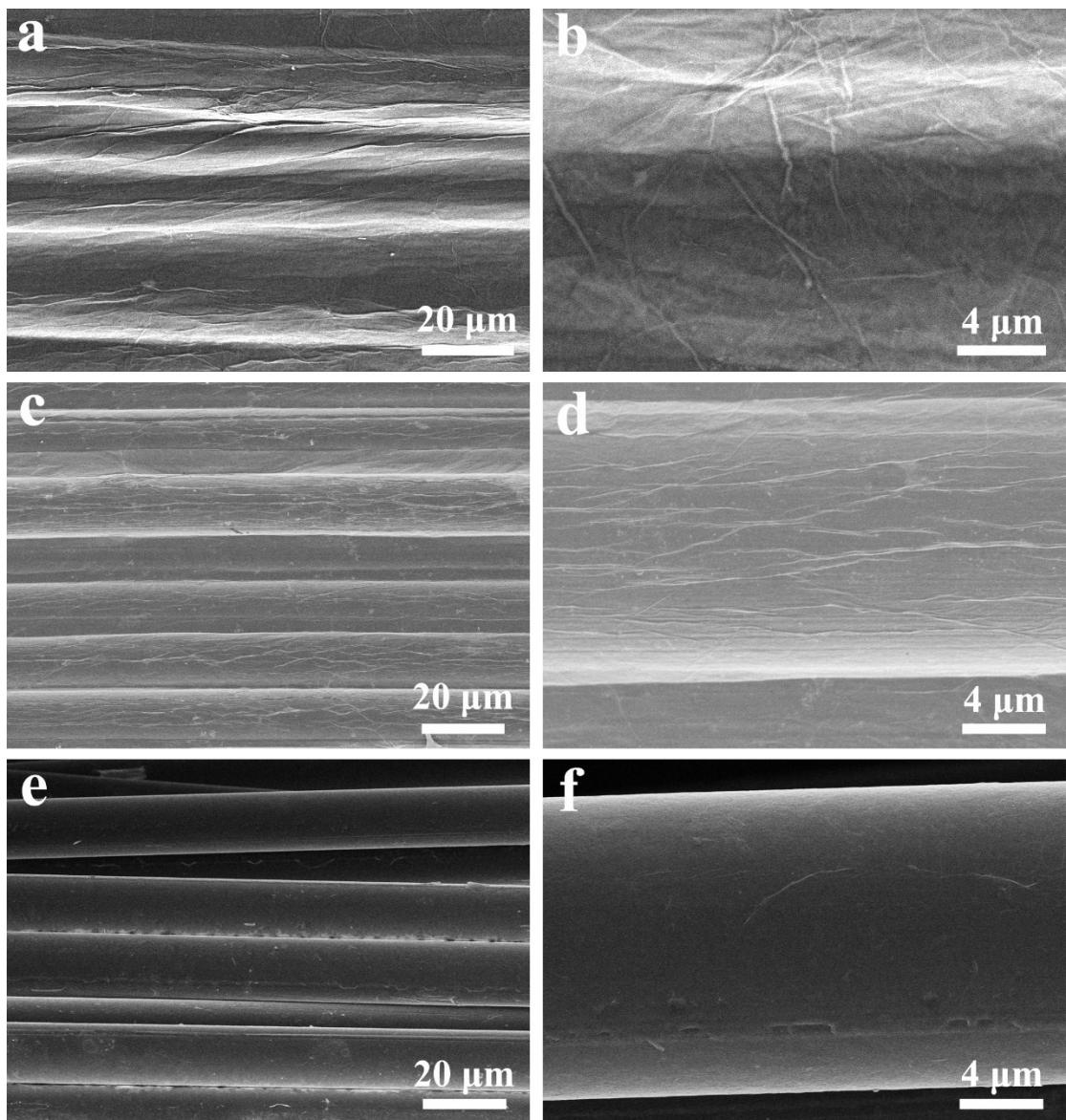
**Figure S3.** SEM images of GrPI@AT yarns experiencing (a-b) 12, (c-d) 7 and (e-f) 2 dipping times.
