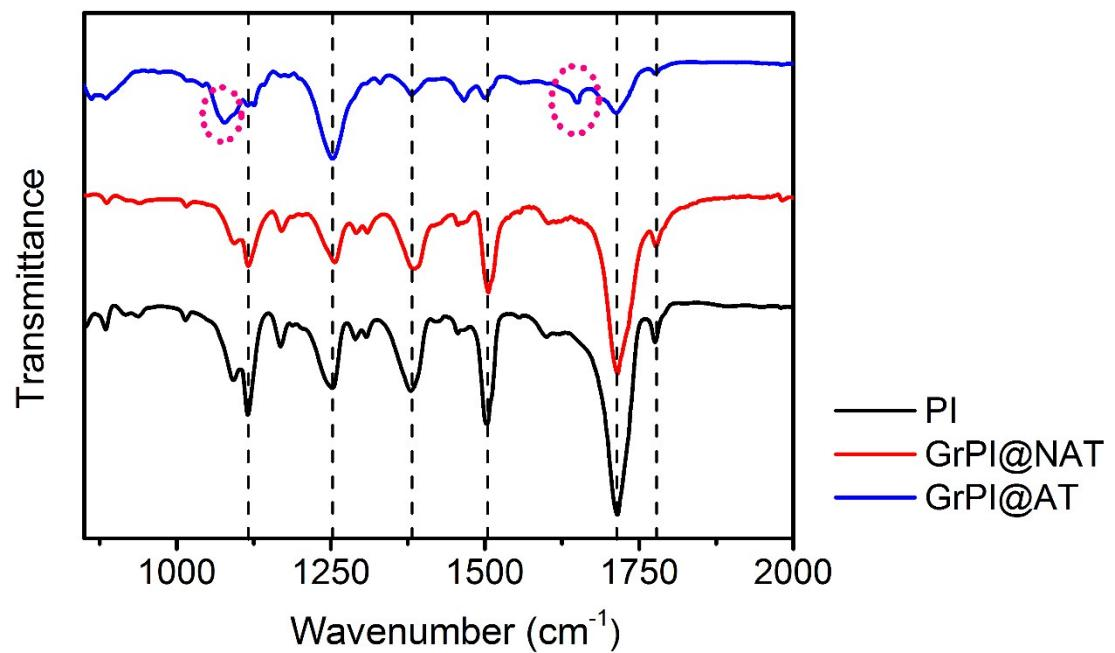
**Figure S5.** FTIR spectra of PI yarn, GrPI@NAT and GrPI@AT yarns.
