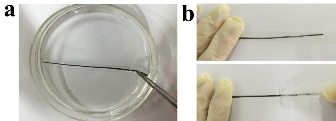
**Figure S9.** **(a)** Clear water after the GrPI@AT yarns underwent water wash. **(b)** Scotch tape test performed on GrPI@AT yarns and clear surface of Scotch tape.
