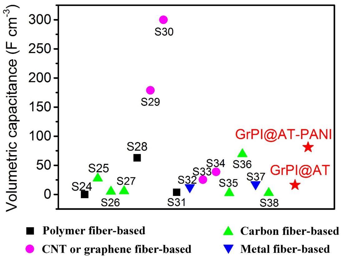
**Figure S13.** Comparison on volumetric specific capacitance between this work and the other supercapacitors based on fibers or textiles.<sup>24-38</sup>
