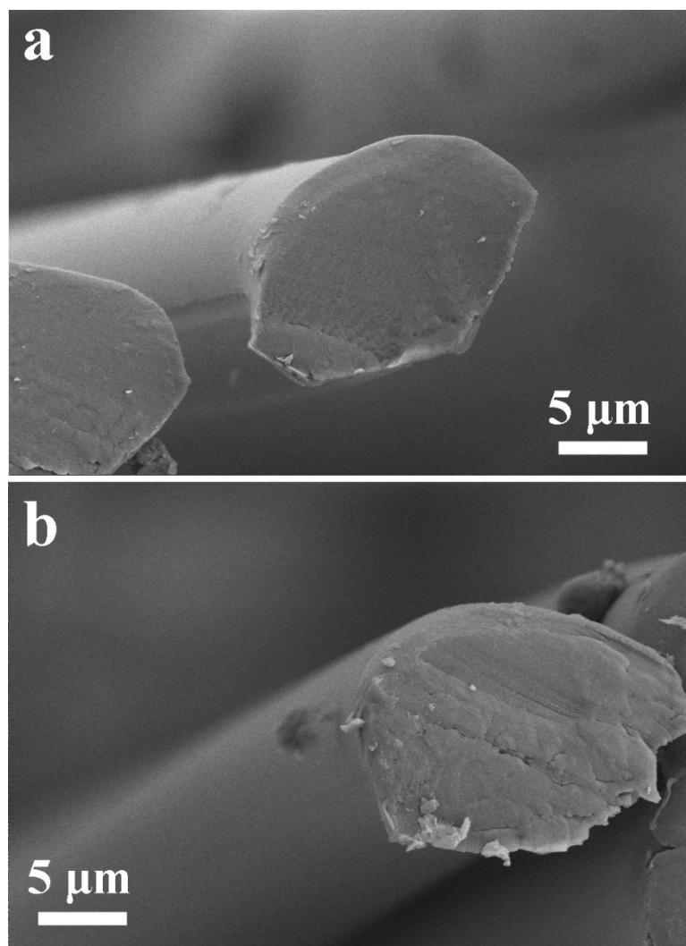
**Figure S2.** Cross-sectional SEM images of (a) non-treated and (b) alkali-treated PI yarns.
