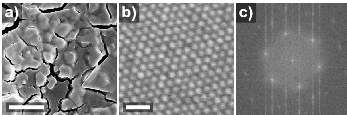
**Figure S2:** a), b) SEM images of samples GNP<sub>5.5 nm</sub>1 shown at two different magnifications and c) the Fourier transform of the SEM image presented in Figure part b). The scale bars are 10  $\mu\text{m}$  in a) and 20 nm in b).
