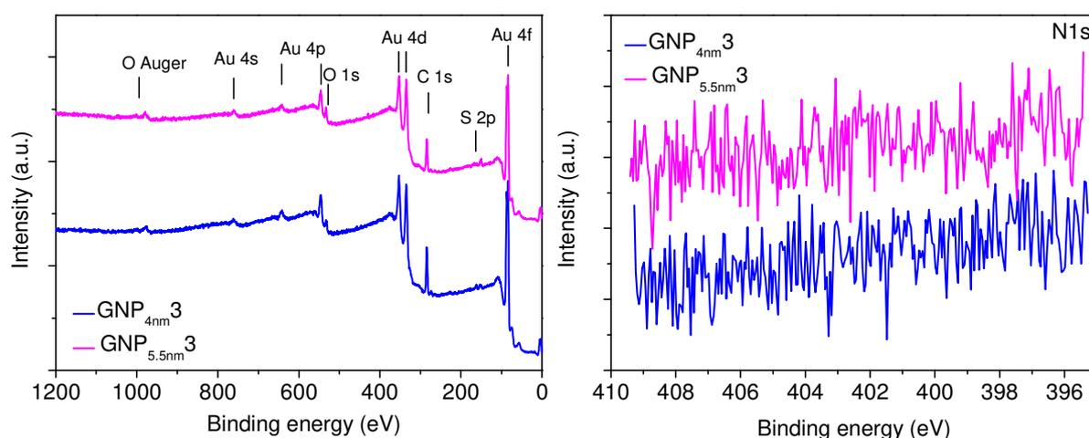
**Figure S1:** XPS spectra (left: survey, right: N region) of GNP superlattice films prepared from sample GNP<sub>4nm</sub>3 (blue) and GNP<sub>5.5nm</sub>3 (magenta). In the survey spectra the expected signals for the elements Au, C and S and some O (due to the exposure to atmosphere prior to the XPS measurements) are observed. The absence of a peak in the energy range between 395 to 410 eV reveals that no nitrogen compounds were detectable.
