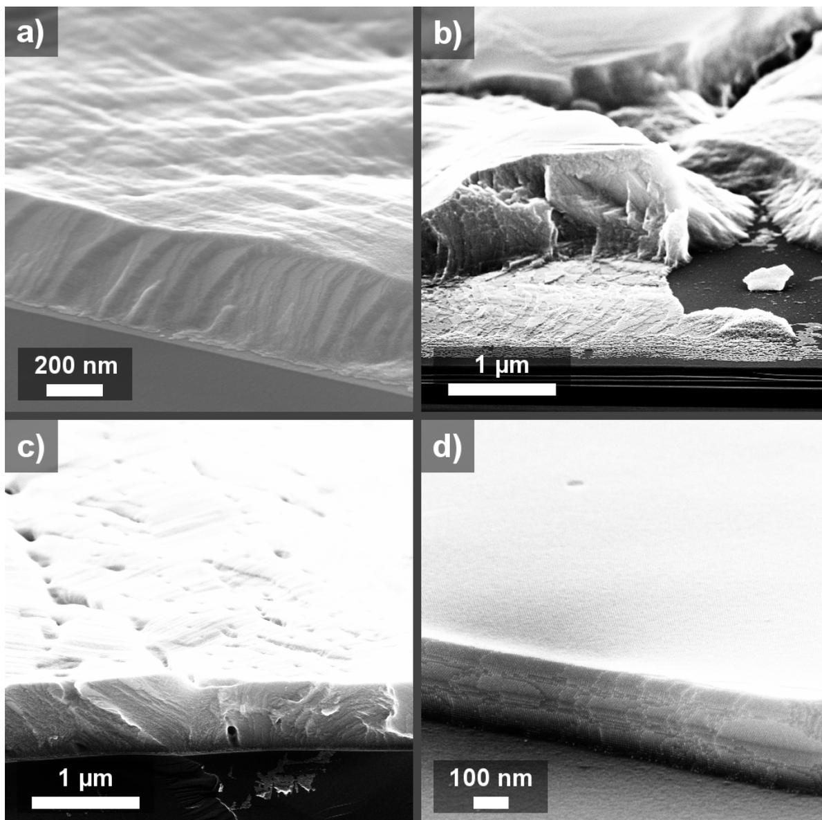
**Figure S3:** Representative SEM images of samples a) GNP<sub>4 nm</sub>1, b) GNP<sub>5.5 nm</sub>1, c) GNP<sub>4 nm</sub>2, and d) GNP<sub>5.5 nm</sub>2 providing cross-sectional views of the cleaved samples.
