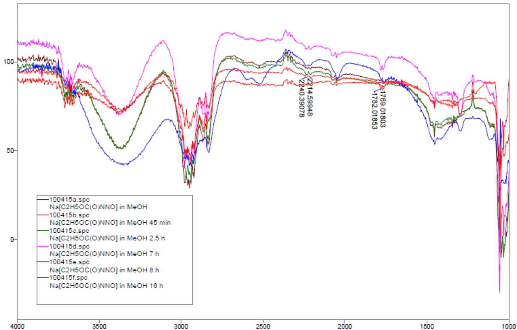
**Figure S10.** Gas-phase IR monitoring of 4-Na in CH<sub>3</sub>OH. Weak bands ( $\nu$ : cm<sup>-1</sup>) 2240, 2214 are from N<sub>2</sub>O (g). Black: Initial; Brown: after 45 min; Green: after 2.5 h; Pink: after 7 h; Blue: after 8 h; Red: after 16 h.
