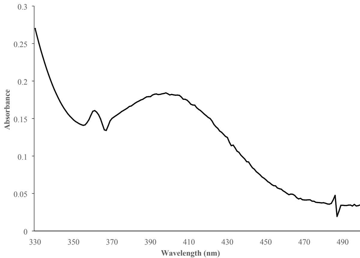
**Figure S5.** UV-vis absorption spectrum of 7.1 mM 4-Na in CH<sub>3</sub>OH.
