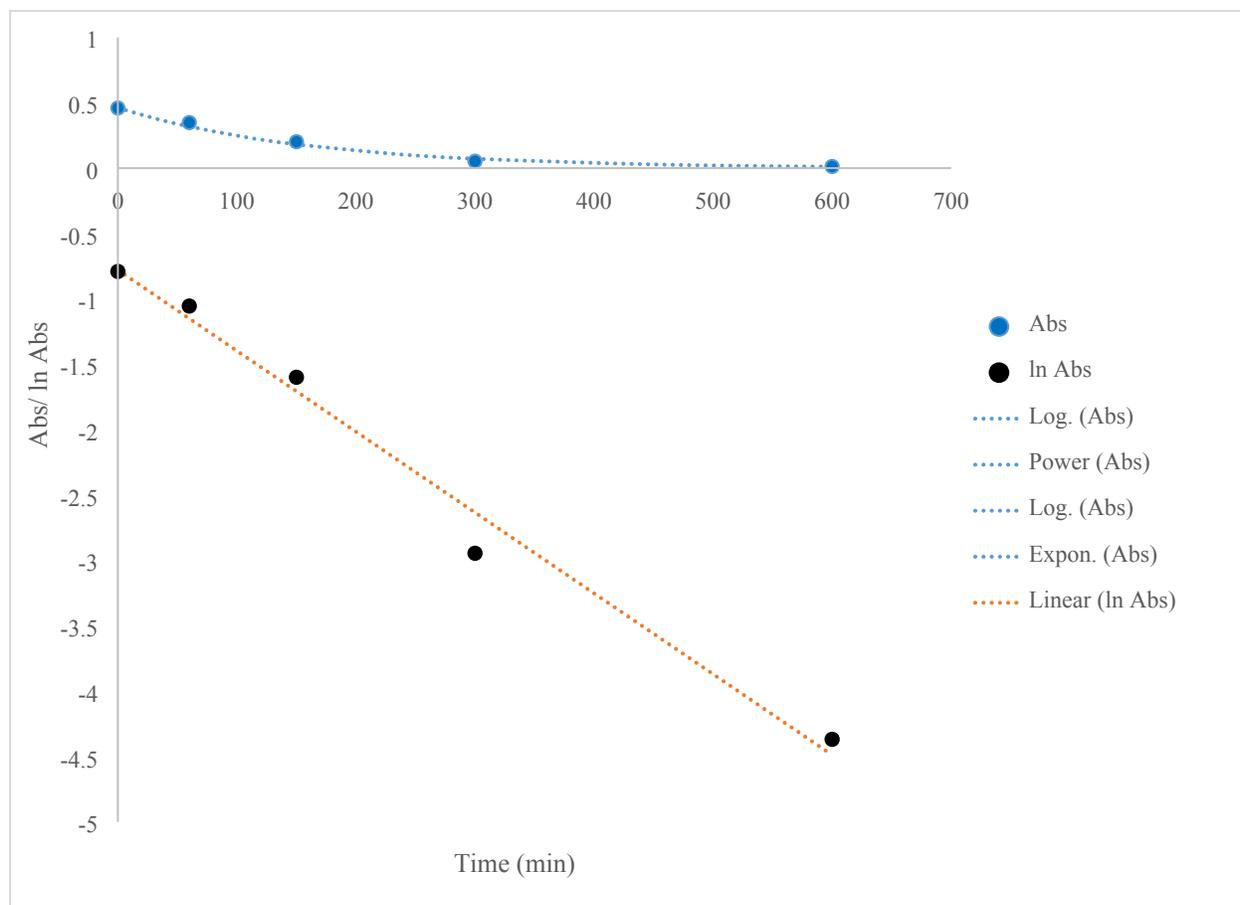
**Figure S12.** UV-vis monitoring at 397 nm of the decomposition of **3-Na** in methanol. Plot of Abs/ln Abs over time (min).
