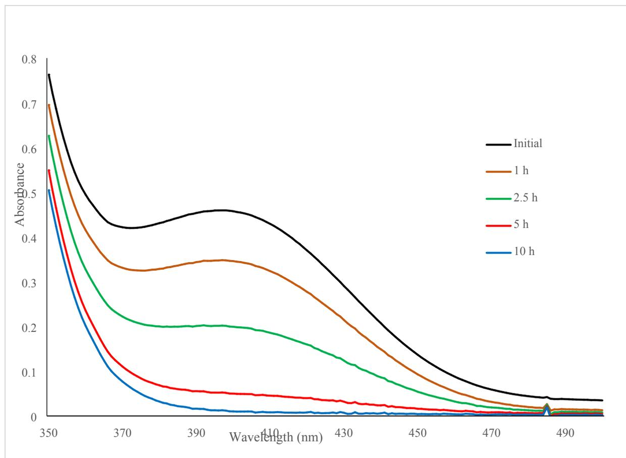
**Figure S11.** UV-vis monitoring spectra of the decomposition of **3-Na** in methanol. Black (initial); Brown (after 1 h); Green (after 2.5 h); Red (after 5 h); Blue (after 10 h).
