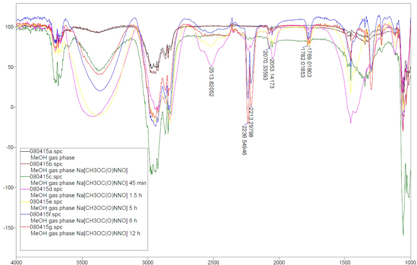
**Figure S9.** Gas-phase IR monitoring of **3-Na** in CH<sub>3</sub>OH. Weak bands ( $\nu$ : cm<sup>-1</sup>) 2240, 2214 are from N<sub>2</sub>O (g). Strong overlap with solvent bands around 1300 cm<sup>-1</sup> prevent identification of N<sub>2</sub>O symmetric band. Black: CH<sub>3</sub>OH; **Brown**: CH<sub>3</sub>OH with **3-Na** initial; **Green**: after 45 min; **Pink**: after 1.5 h; **Yellow**: after 5 h; **Blue**: after 6 h; **Red**: after 12 h.
