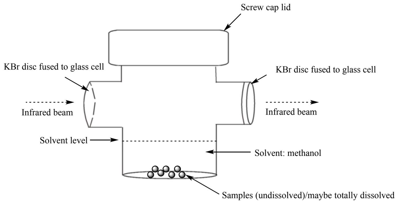
**Figure S16.** Diagram of custom-made IR gas cell.
