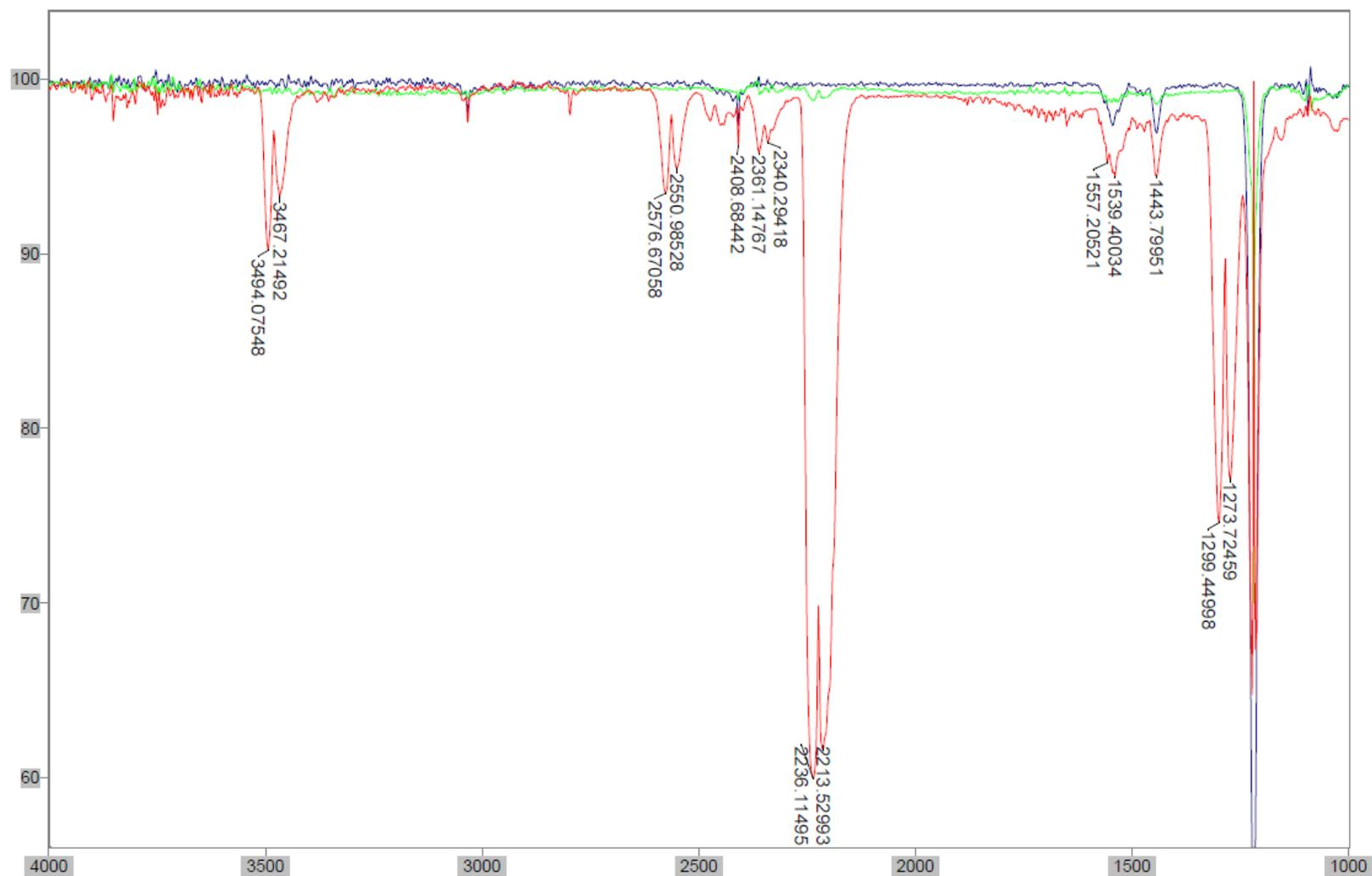
**Figure S8.** Gas-phase IR monitoring of decomposition of nitramide ( $\text{H}_2\text{NNO}_2$ ) using  $\text{K}_2\text{CO}_3$  in  $\text{CHCl}_3$ . Bands ( $\nu$ :  $\text{cm}^{-1}$ ): 2236, 2214 (asymm) and 1299, 1274 (sym) are from  $\text{N}_2\text{O}$  (g). **Green:**  $\text{CHCl}_3$ ; **Blue:**  $\text{H}_2\text{NNO}_2$ ; **Red:**  $\text{H}_2\text{NNO}_2$  with  $\text{K}_2\text{CO}_3$ .
