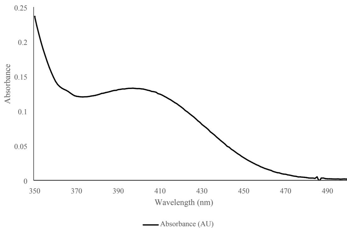
**Figure S4.** UV-vis absorption spectrum of 3.4 mM **3-Na** in CH<sub>3</sub>OH.
