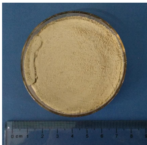
Figure S1 Digital photograph of the as-prepared monolithic NiO aerogel.
