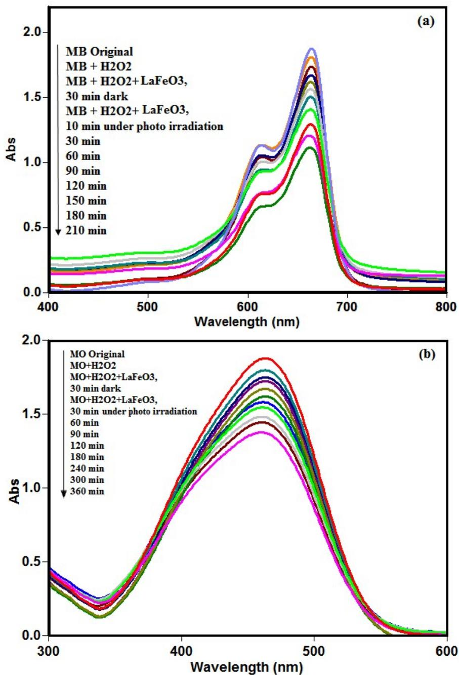
**Fig. S1.** UV-Vis time dependent absorption spectrum during photocatalytic reaction of MB (a) and MO (b) in the presence of LaFeO<sub>3</sub> nanoparticles (concentration of MB and MO= 25 mg/L, amount of catalyst = 20 mg, 2 mL of hydrogen peroxide 0.1 M, reaction temperature =32°C).
