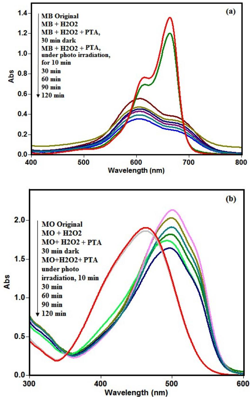
**Fig. S2.** UV-Vis time dependent absorption spectrum during photocatalytic reaction of MB (a) and MO (b) in the presence of PTA (concentration of MB and MO= 25 mg/L, amount of catalyst = 10 mg, 2 mL of hydrogen peroxide 0.1 M, reaction temperature =32°C).
