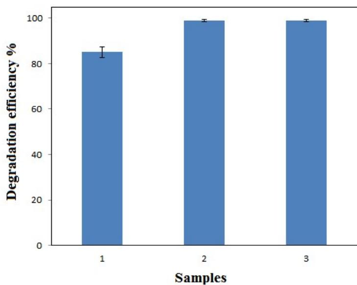
**Fig. S3.** Effect of different amounts of hydrogen peroxide on the photocatalytic degradation of MB in the presence of composite catalyst. concentration of MB= 25mg/L, amount of catalyst = 25 mg, amount of hydrogen peroxide addition, 1 mL (sample 1), 2mL (sample 2), 3 mL (sample 3), reaction temperature =32°C).
