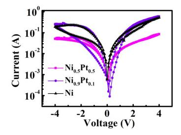
Fig. S1 I-V characteristics of Au/Ni $_x$ Pt $_{(1-x)}$  NPs/NSTO/In devices.
