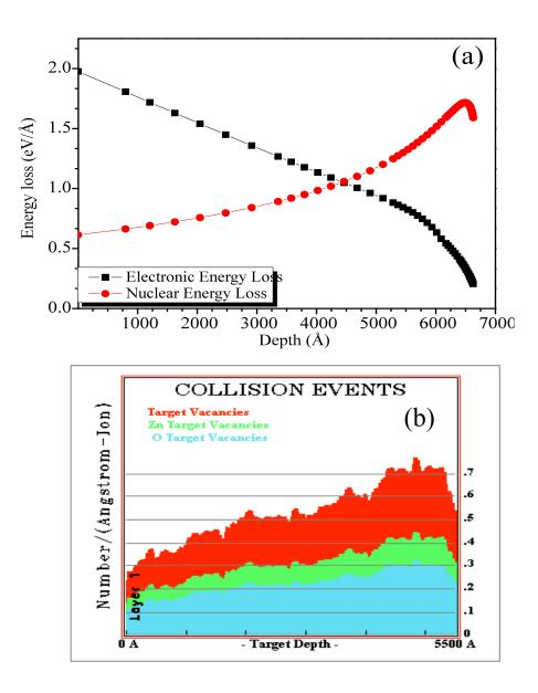
**Fig. 1**: (Color online) (a) Electronic and Nuclear energy losses with penetration depth of 800 keV Ar ions in Zn<sub>0.95</sub>Mn<sub>0.05</sub>O films, calculated from SRIM. (b) Vacancy created by ion beam throughout the depth of the films, calculated from SRIM.
