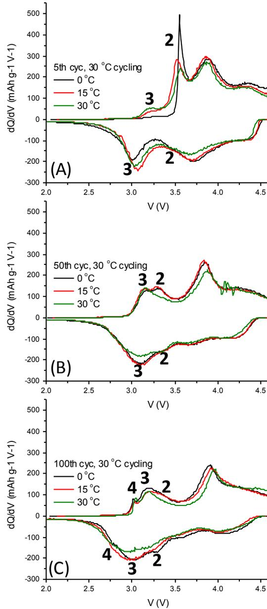
Figure S 3: Differential capacity vs. voltage plots of the Li-rich material electrodes activated at 0 – 30 °C, cycled at 30 °C, over 100 cycles.
