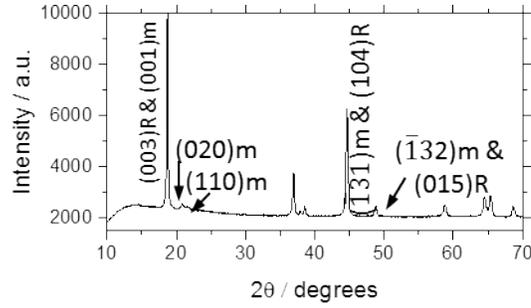
Figure S 2: XRD pattern from pristine, uncycled Li-rich  $0.35\text{LiMn}_2\text{O}_3 \cdot 0.65\text{Li}[\text{Mn}_{0.45}\text{Ni}_{0.35}\text{Co}_{0.20}]\text{O}_2$  powder with some reflections indicated.
