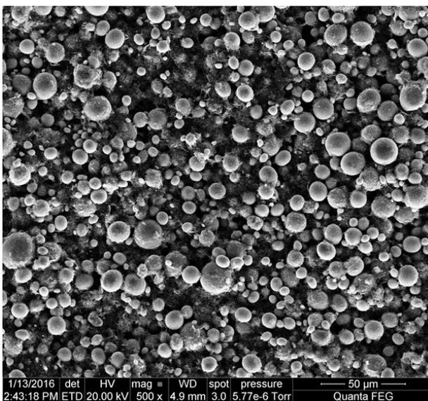
Figure S 1: SEM micrograph of an uncycled  $0.35\text{LiMn}_2\text{O}_3 \cdot 0.65\text{Li}[\text{Mn}_{0.45}\text{Ni}_{0.35}\text{Co}_{0.20}]\text{O}_2$  electrode.
