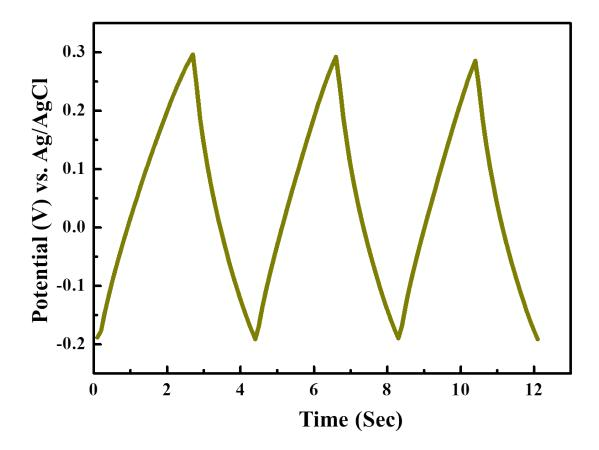
Fig. S3 Galvanostatic charge/discharge behavior of pure MnS (Expanded image of Fig. 11)
