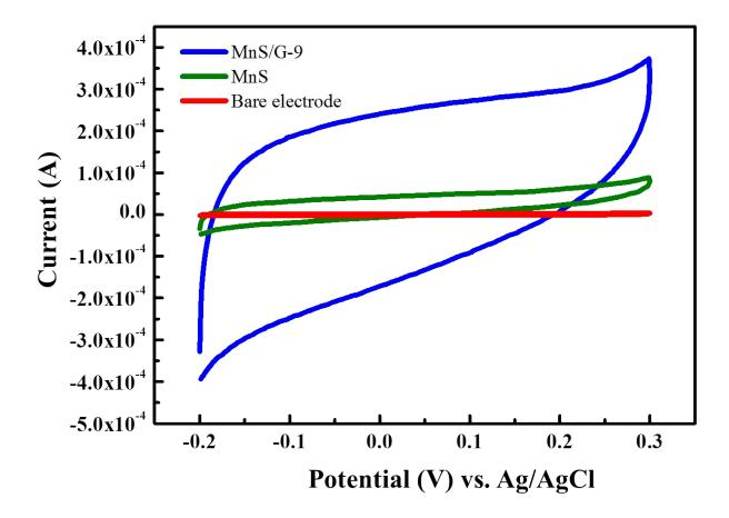
Fig. S2 Comparison of CV curve of bare carbon electrode, MnS/G-9 and pure MnS at 100 mV scan rate
