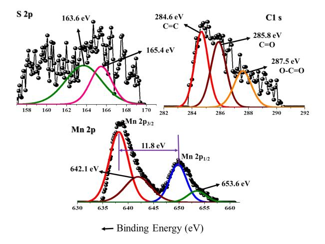
Fig. S1 Core level XPS spectrum of S2p, C1s and Mn2p of MnS/G-9 nanocomposite
