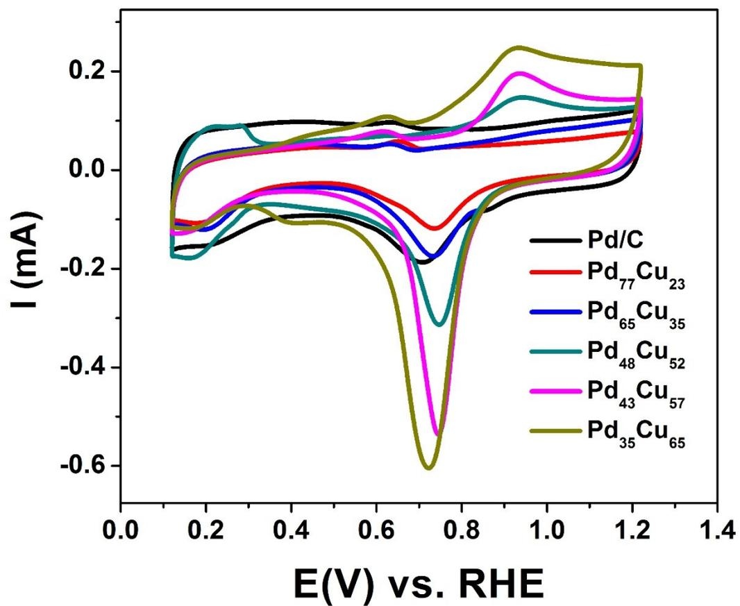
**Figure. S2** Cyclic voltammograms (CVs) of the five PdCu/C catalysts and commercial Pd/C in an Ar-saturated 0.1 M KOH solution at a sweep rate of 50 mV/s
