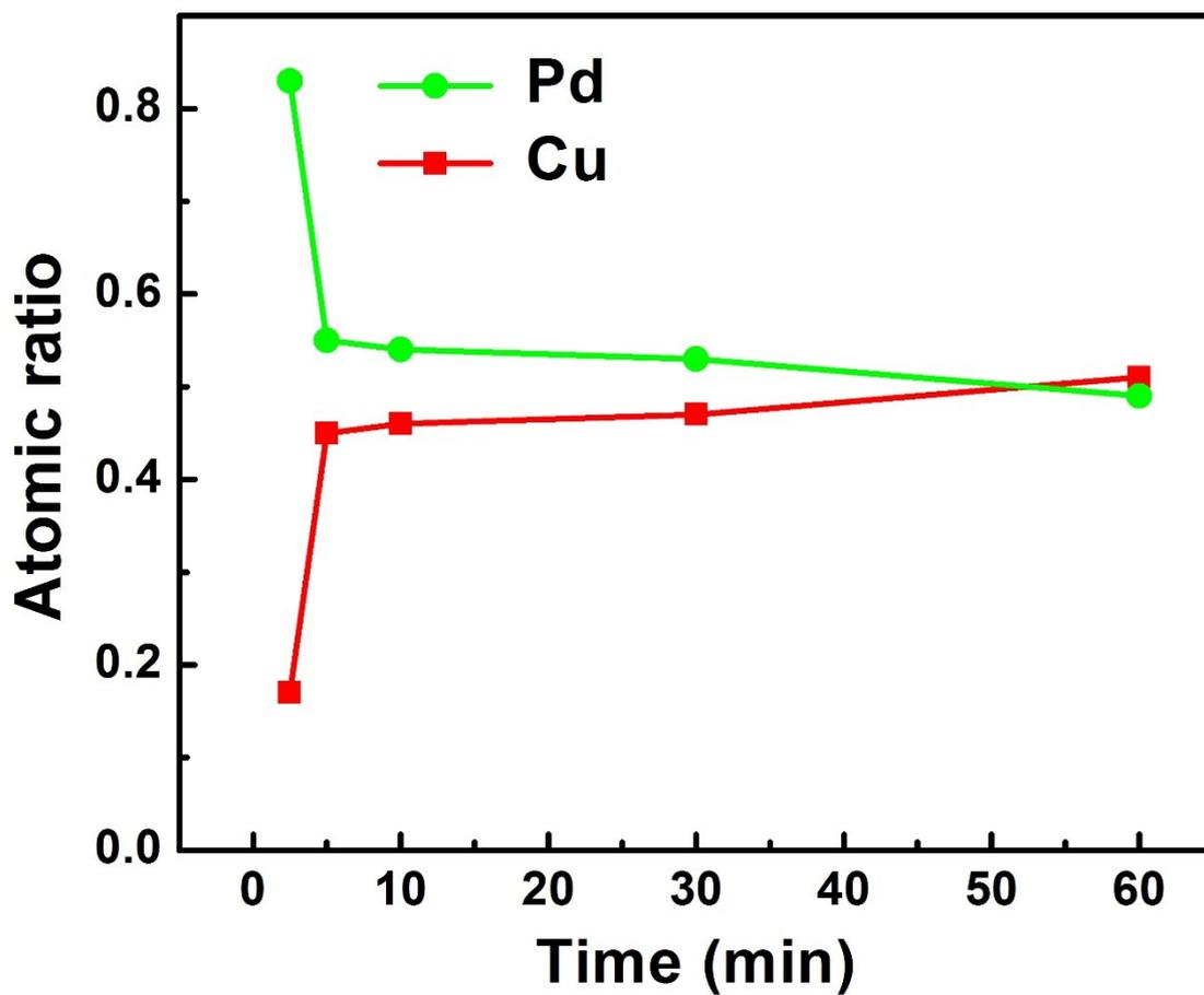
**Figure. S1** ICP-AES data of the PdCu nanostructures prepared using the standard procedure, except for different period of the reaction from 2.5 to 5, 10, 30 and 60 min.
