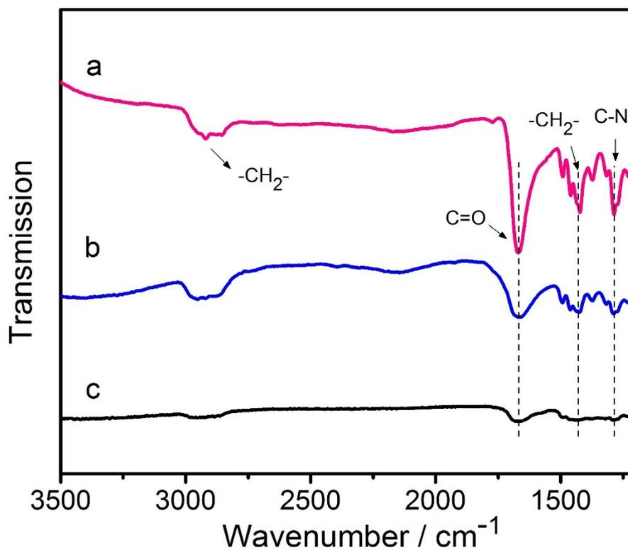
**Figure. S3** FTIR spectra of the  $\text{Pd}_{48}\text{Cu}_{52}$  nanodendrites treated by different treatment methods. The  $\text{Pd}_{48}\text{Cu}_{52}$  nanodendrites (a) were washed by alcohol for one time, (b) were washed by alcohol for four times, and (c) were treated by tert-butylamine and  $\text{NaBH}_4$  and washed by alcohol for three times.
