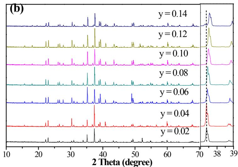
**Fig. S1.** XRD patterns of  $\text{La}_{1-x}\text{Si}_3\text{N}_5:\text{xCe}^{3+}$  ( $x=0.03, 0.06, 0.09, 0.12, 0.15, 0.18, 0.21$ ) samples (a) and  $\text{La}_{1-y}\text{Si}_3\text{N}_5:\text{yCe}^{3+}$  ( $y=0.02, 0.04, 0.06, 0.08, 0.10, 0.12, 0.14$ ) samples (b).
