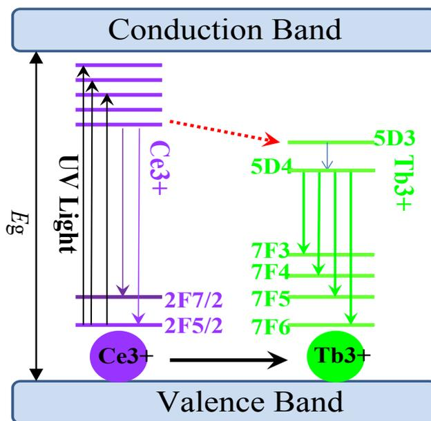
**Fig. S2.** Illustration of the ET models for  $\text{Ce}^{3+}-\text{Tb}^{3+}$  in the  $\text{LaSi}_3\text{N}_5$  host.
