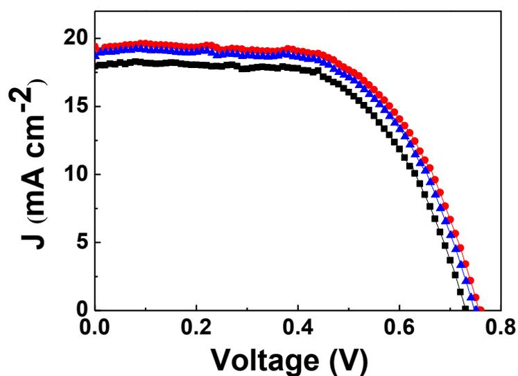
**Fig. S3** J-V curve of Cell B on the 1<sup>st</sup> day (—■—), 30<sup>th</sup> day (—●—) and 120<sup>th</sup> day (—▲—) testing under the simulated AM 1.5 solar spectrum irradiation at 100 mW cm<sup>-2</sup>. The Cell was tested using an aluminum foil mask with an aperture area of 0.1 cm<sup>2</sup>.
