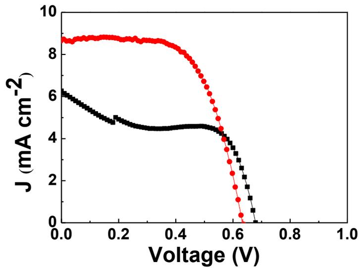
**Fig. S1** The  $J$ - $V$  curves of Cell A' (—■—) and Cell B' (—●—) under the simulated AM 1.5 solar spectrum irradiation at  $100 \text{ mW cm}^{-2}$ . Cells were tested using an aluminum foil mask with an aperture area of  $0.1 \text{ cm}^2$ . Poor fill factor (FF) and low efficiency of the devices were obtained.
