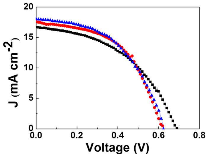
**Fig. S2** The  $J$ - $V$  curves of Cell C (—■—), Cell D (—●—) and Cell E (—▲—) under the simulated AM 1.5 solar spectrum irradiation at  $100 \text{ mW cm}^{-2}$ . Cells were tested using an aluminum foil mask with an aperture area of  $0.1 \text{ cm}^2$ .
