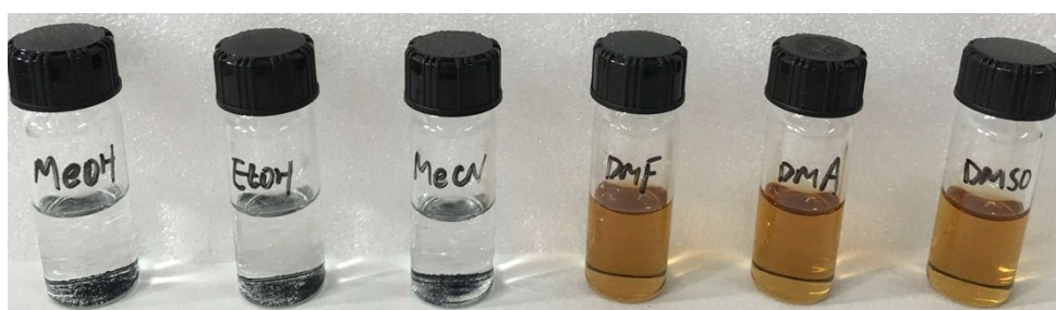
Figure S7. Freshly as-prepared crystals of 2 can be insoluble in MeOH, EtOH, MeCN, but readily dissolve in DMF, DMA and DMSO.
