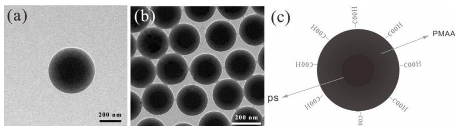
Figure S1: a) and b) TEM image of the P(St-MMA-AA) NPs. c) Schematic diagram of the P(St-MMA-AA) NPs.
