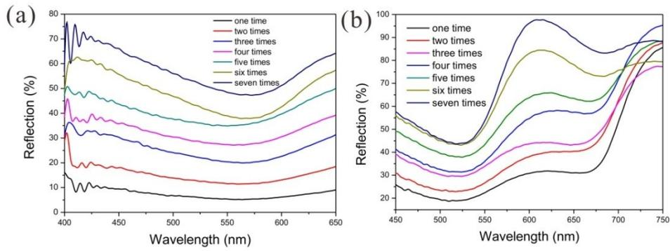
Figure S4: Reflectance spectrum of the violet a) and red b) coated fabrics with different spraying times.
