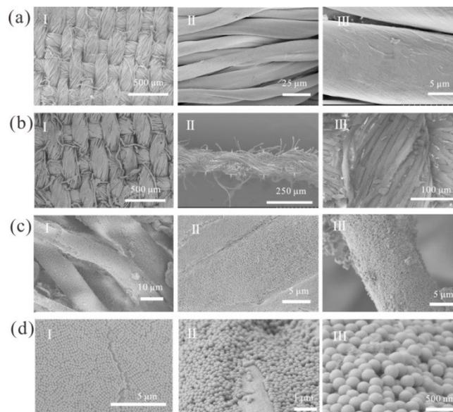
Figure S3: a I )-aIII) The surface morphology of original fabric and fibers. b I )-bIII) The surface and section morphology of the coated fabric. c I )-cIII) The particles were attached on the surface of each fiber. d) Array of the particles on the fibers.
