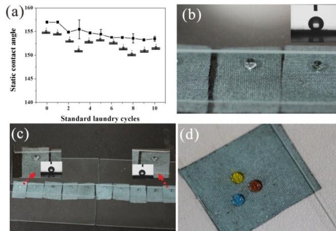
Figure S10: a) The water CA of the coated fabric after 10 cycles of standard machine laundry. b) Optical image of the superhydrophobic coated fabrics. c) The coated fabrics maintained superhydrophobicity after 10 cycles of standard machine laundry. d) Three 6  $\mu$ l water droplets coloring with different dyes became spherular.
