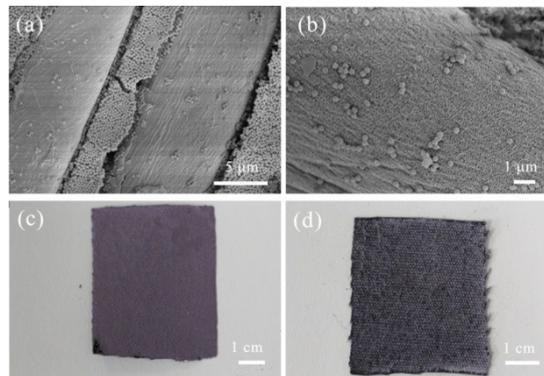
Figure S6: a), b) Particles on the coated fabrics without incorporation of PA nearly fell off the fiber surface after a cycle. c), d) Without incorporation of PA, the fabric was faded badly after a laundry cycle (left: before washing, right: after washing).
