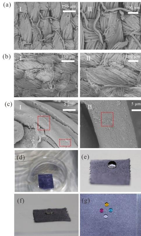
Figure S11: The SEM of supersonic vibration treated fabrics and optical image of superhydrophobic coated fabric after ultrasonic washing. a I ) and a II )SEM images of original coated fabrics. b I ) and b II )SEM images of coated fabrics treated by ultrasonic washing. c I ) and c II ) Morphology of fibers after supersonic washing.. d) The process of supersonic washing. e)-g) Optical images of superhydrophobic coated fabric at different angle view.
