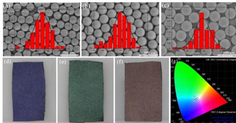
Figure S2: a)-c) SEM image and particle size distribution of the P(St-MMA-AA) NPs. d)-f) Optical images of spray coated fabrics with nanoparticle diameter of 217nm (d), 257nm (e), and 294 nm (f), respectively. g) The different reflection colors of the nanoparticles in Commission Internation de l' Eclairage (CIE) chromaticity values: square (voilet), circle (green) and triangle (red).
