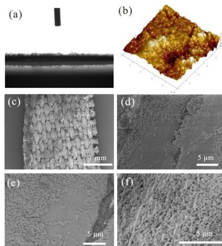
Figure S12: a) Static contact angle of the fabrics and b) the AFM Image of coated fabrics by plasma treatment. c) Morphology of coated fabrics by plasma treatment. d)-f) Most of particles fell off the fibers by plasma treatment.
