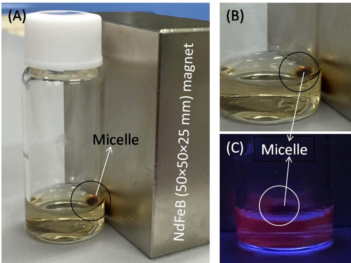
**Fig.S3** Micelles under an external magnetic field. (A, B) Micelles under illumination with white light and 365-nm UV light (C).
