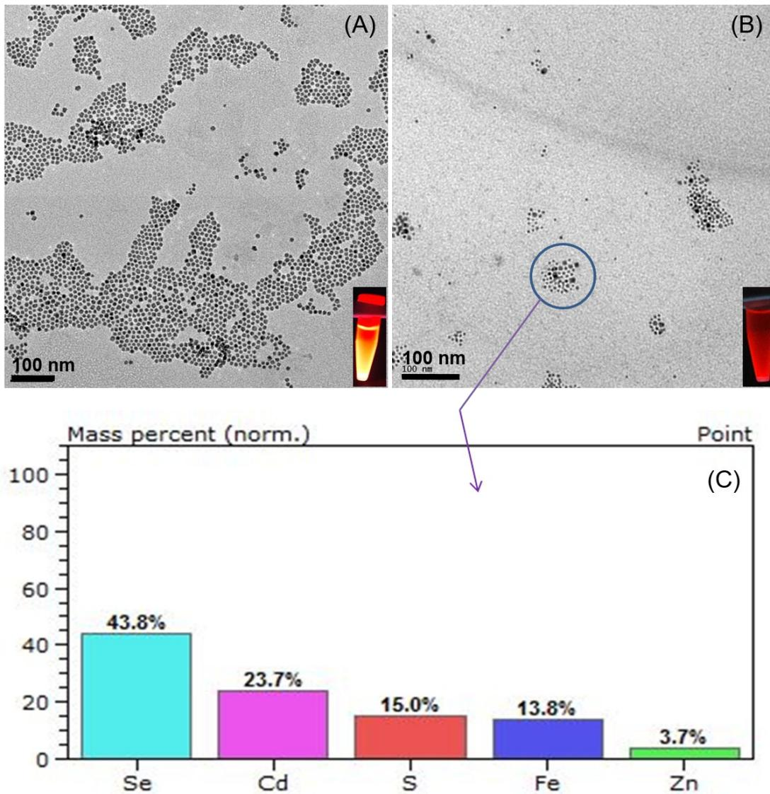
**Fig.S2** (A) TEM micrograph of CdSe/ZnS QDs in chloroform.(B) Micelles [CdSe/ZnS + Fe<sub>3</sub>O<sub>4</sub> NPs] in HPLC water. (C) Elemental analysis of micelles. (Inset A, B: Fluorescence emissions of the samples under UV light excitation)
