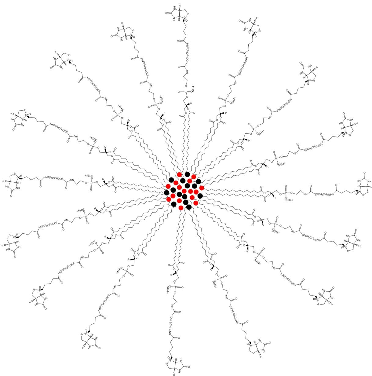
**Fig.S1** Structure of micelle. CdSe/ZnS QDs (red dots) and Fe<sub>3</sub>O<sub>4</sub> NPs (black dots) coencapsulated in a phospholipid [DSPE-PEG (2000)-biotin] micelle.
