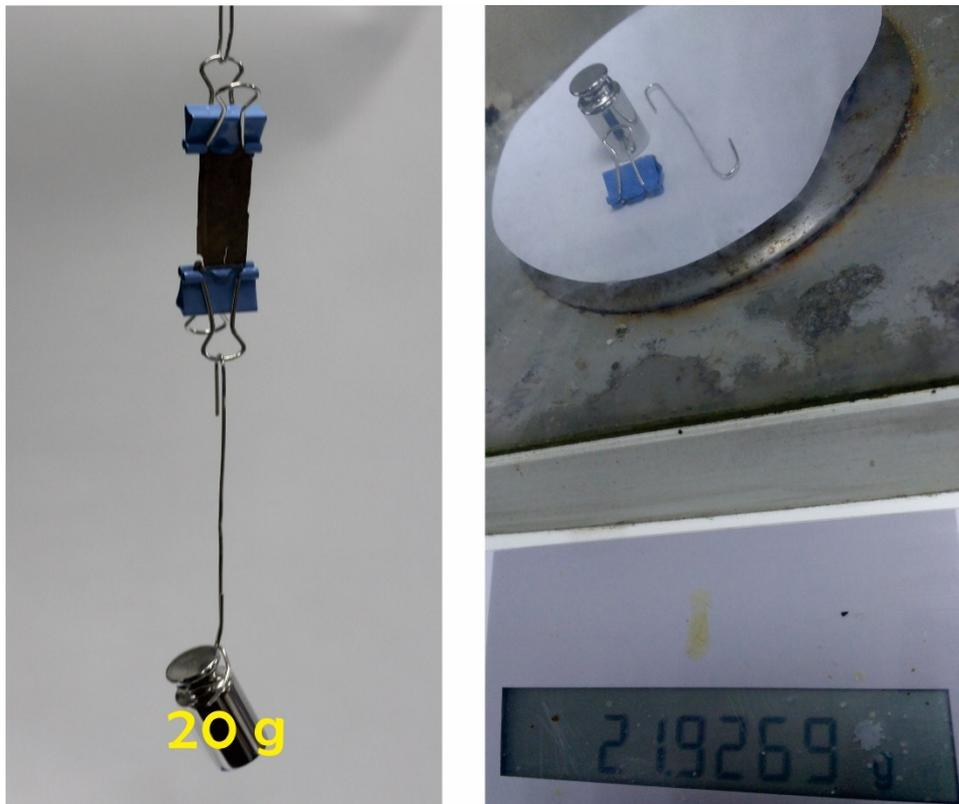
**Figure S8.** Digital pictures of the mechanical testing of the F-CGO3 membrane by overhanging weight.
