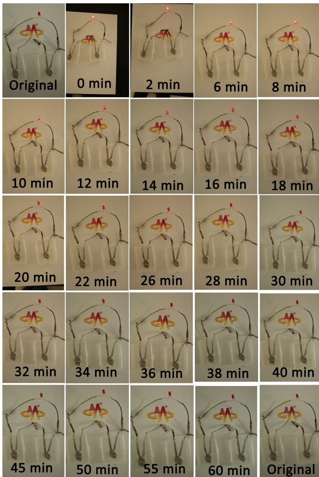
Fig. S3. The LED lighted by two supercapacitors in series at different time.
