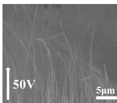
Fig. S2 Cross-sectional SEM images of the upper part of 50V upward after field emission test.
