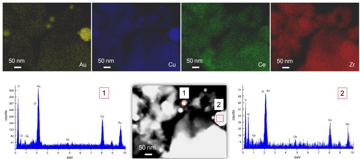
**Figure S2.** STEM images and EDX spectra of CuAu/CeZrO<sub>x</sub>(1:1).
