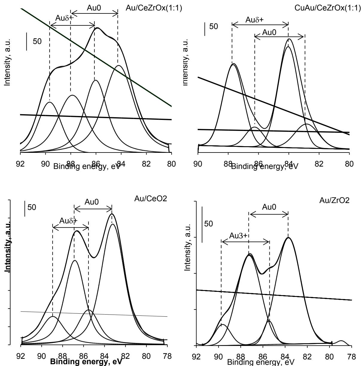
**Figure S3.** XP spectra of Au 4f region recorded for selected catalysts.
