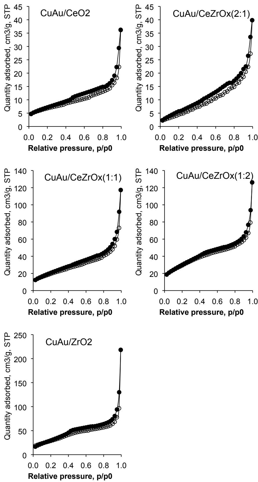
**Figure S1.** The nitrogen adsorption/desorption isotherms for selected catalysts.
