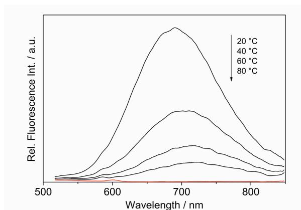
**Figure S2.** Emission spectra of **4b** ( $c = 2.5 \mu\text{M}$ , with 0.25% v/v DMSO) in glycerol (black lines) and in phosphate buffer ( $c_{\text{Na}^+} = 16 \text{ mM}$ , pH 7.0) at 20 °C (red line);  $\lambda_{\text{ex}} = 500 \text{ nm}$ . The arrow indicates the change in emission intensity with increasing temperature.
