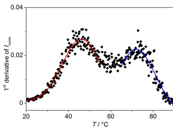
**Figure S4.** First derivative of the normalized change in emission intensity (Figure S3 D1) at  $LDR = 1.3$ . The red and the blue line represent the best fit according to the Gaussian function of the first maximum at  $T_m \approx 46$  °C and of second maximum at  $T_m \approx 72$  °C, respectively.
