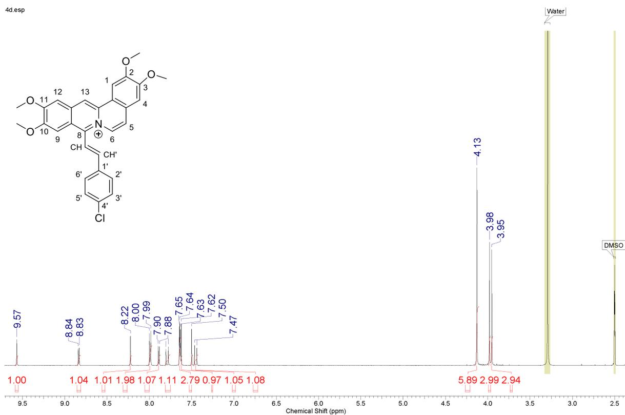
**Figure S12.** <sup>1</sup>H-NMR spectrum (600 MHz) of (E)-8-(4'-chlorostyryl)coralyne tetrafluoroborate (4d) in DMSO-*d*<sub>6</sub>.
