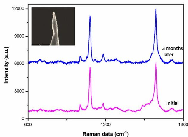
**Figure S2.** SERS spectrum of the same Au NTNP at (a) initial time and (b) 3 months later by using  $10^{-3}$  mol/L 4-MBA solution as probe molecule. The inset is the SEM of the Au NTNP with the apex diameter about 80 nm.
