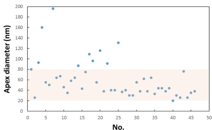
**Figure S1.** Distribution diagram of the apex diameters of the Au NTNPs prepared in the experiment, in which 79% Au NTNPs (plots with yellow background) are with apex diameter between 30 nm to 80 nm.
