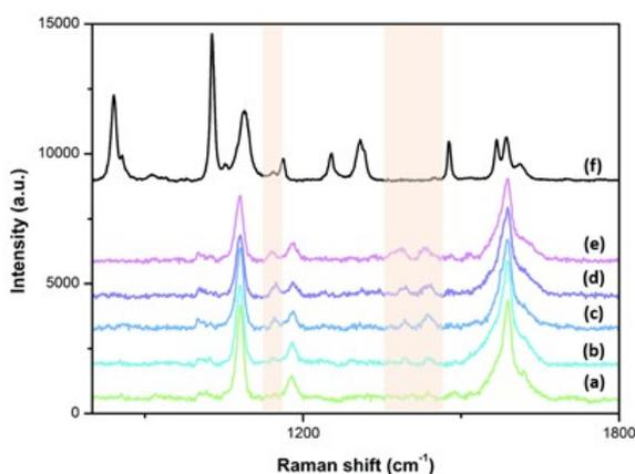
**Figure S3.** SERS spectrum of  $10^{-3}$  mol/L PATP absorbed on Au NTNP substrate immediately after the preparation of the PATP ethanol solution with laser exposure after (a) 10s (b) 40s (c) 50s (d) 70s (e) 80s; (f) Normal Raman spectrum of PATP powder.
