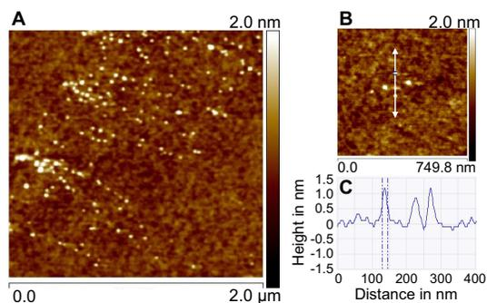
Figure S 1: The GQDs deposited on  $\text{SiO}_2$  as seen by an atomic force microscope. Their apparent width is  $\approx 20$  nm, which is much larger than their true width, in accordance with earlier works. The height of less than 1 nm indicates single-layer graphene.
