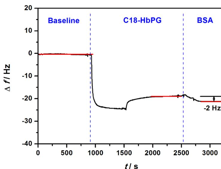
**Fig. S5** Changes in the resonance frequency ( $\Delta f$ ) of the QCM sensor crystal over time.
