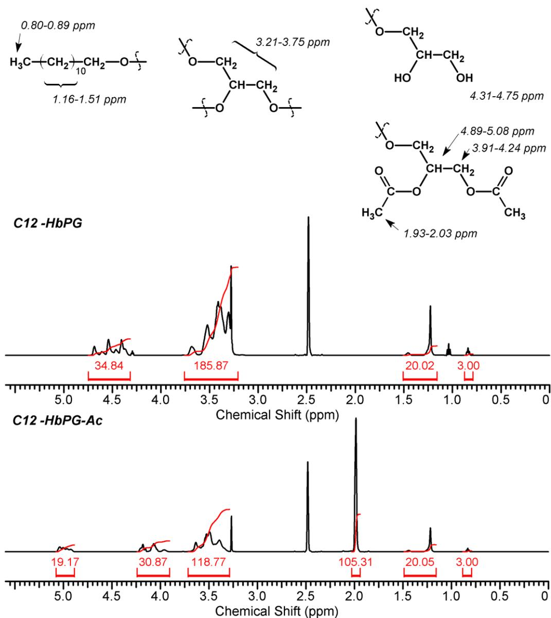
**Fig. S1** <sup>1</sup>H NMR spectra of C12-HbPG (top) and its acetyl derivative (bottom) in DMSO-*d*<sub>6</sub>.
