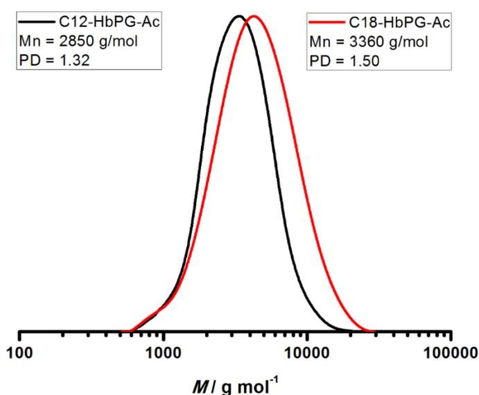
**Fig. S3** Molecular weight distribution curves of acetyl derivatives of HbPG samples.
