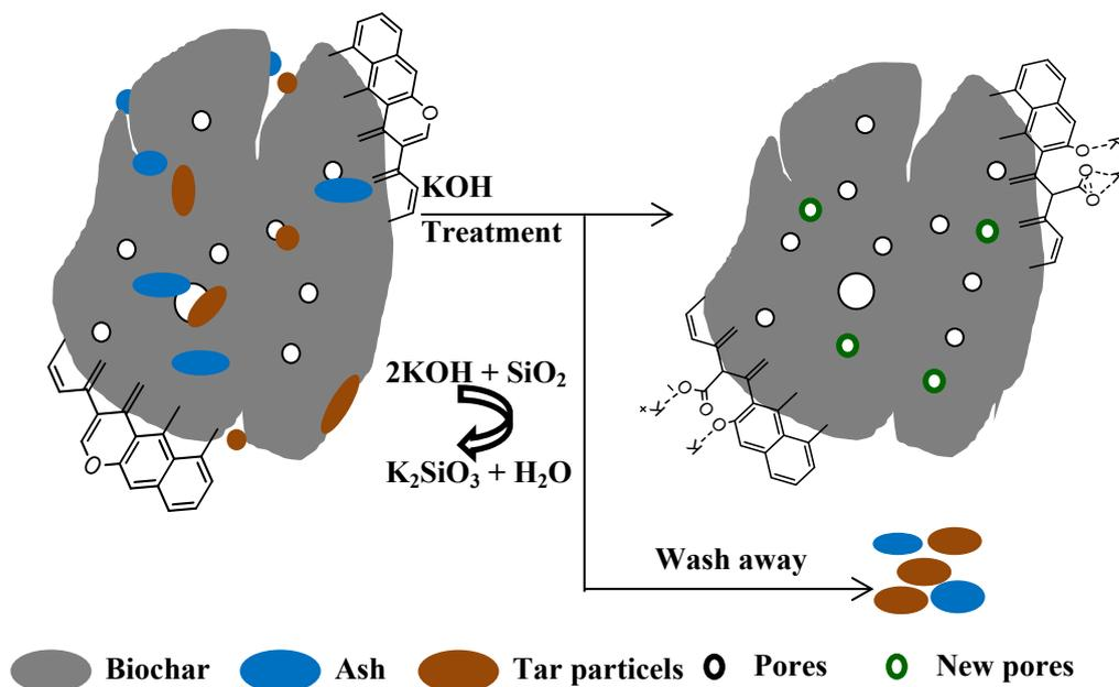
**Figure S1.** Schematic diagram of KOH modifying processes. **KOH modifying**
