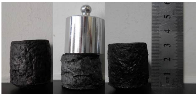
Fig. S6- Compression and recovery picture of GCHA-20. The weight is 200g.
