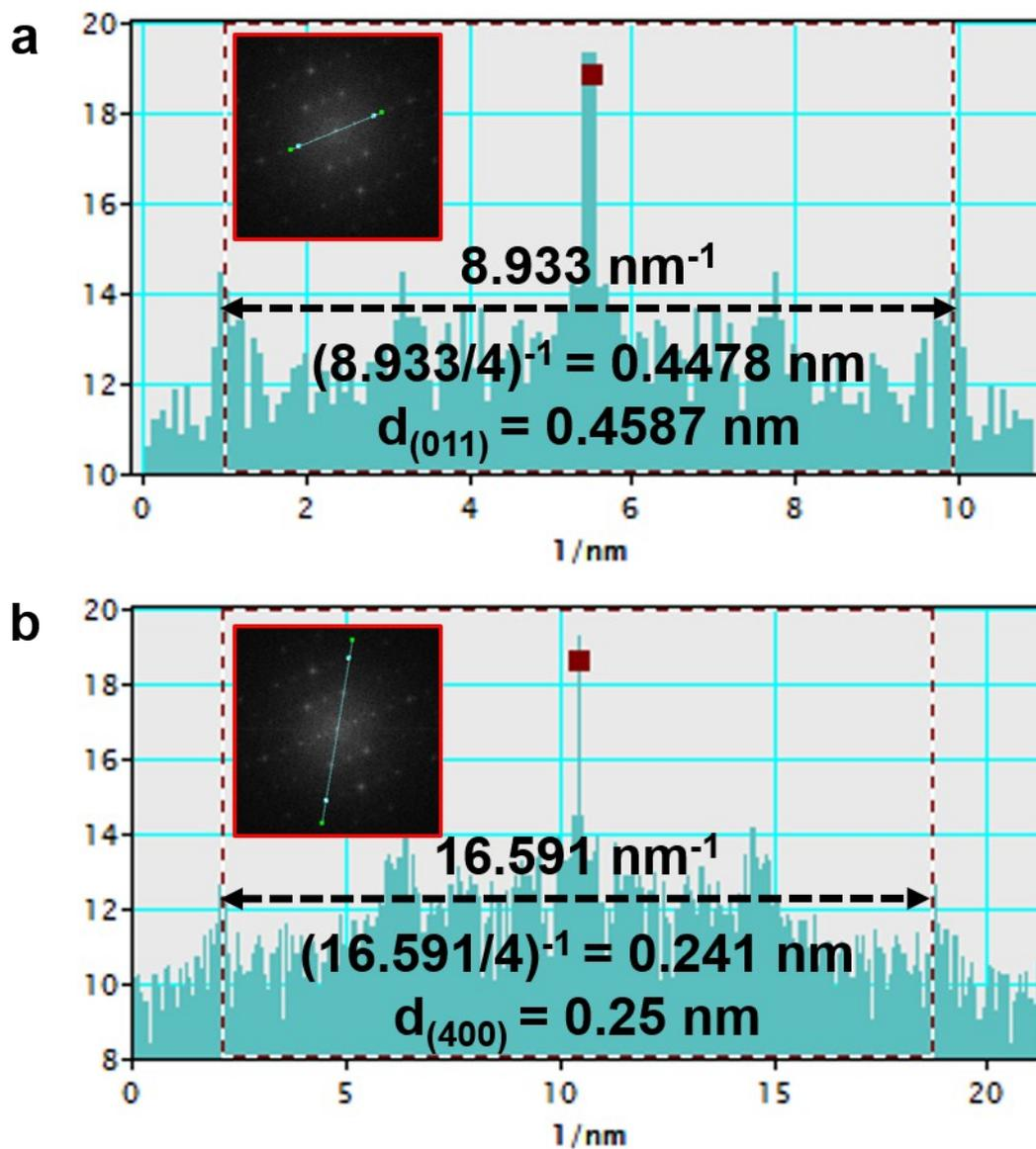
Fig. S2 (a) The distance between (011) reciprocal points of Al<sub>2</sub>Se<sub>3</sub>. (b) The distance between (400) reciprocal points of Al<sub>2</sub>Se<sub>3</sub>.
