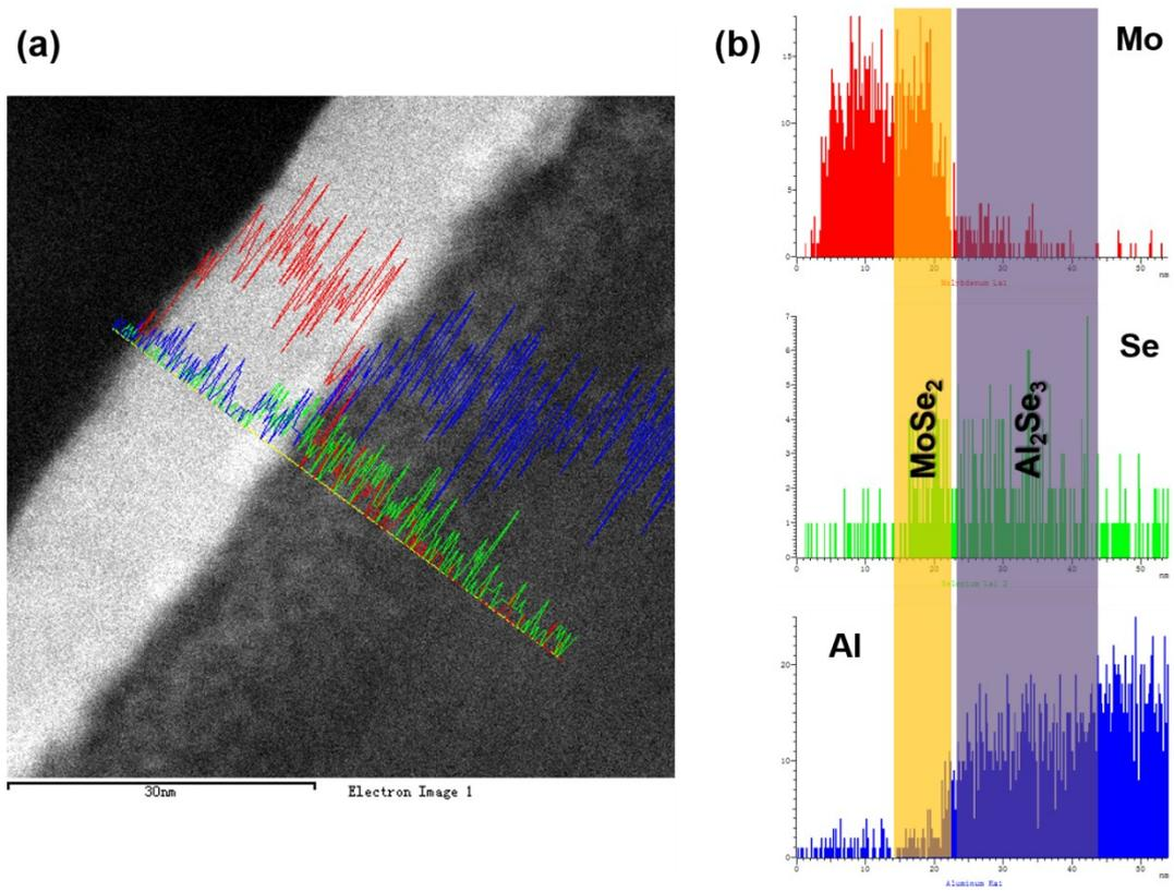
Fig. S1 (a) STEM dark-field image of the MoSe<sub>2</sub>/Al<sub>2</sub>Se<sub>3</sub>/sapphire layer structure. (b) Depth concentration distribution of Mo, Se, and Al.
