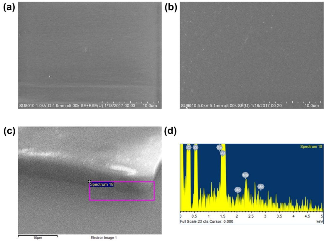
Fig. S3 (a) The top-view SEM image of pristine sapphire. (b) The top-view SEM image of Mo film on sapphire. (c) The tilt-view SEM image of the patterned MoSe<sub>2</sub>/Al<sub>2</sub>Se<sub>3</sub> on sapphire. (d) The EDS spectrum of the area corresponding to the rectangle in (c).
