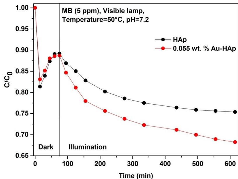
**Figure S2.** Photocatalytic degradation of MB by HAp and 0.055 wt. % Au-HAp catalyst at 50°C under visible light irradiation.
