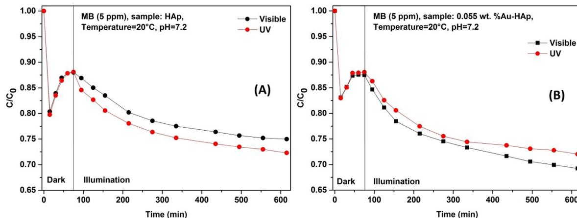
**Figure S1.** Photocatalytic degradation of MB by (A) HAp and (B) 0.055 wt. % Au-HAp catalyst under UV and visible light irradiation.
