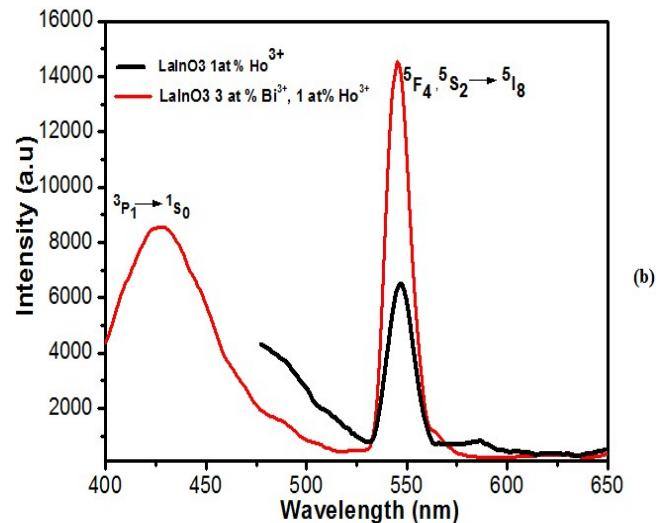
**Fig.4 Emission spectra of Single doped Sm<sup>3+</sup> and Ho<sup>3+</sup> in LaInO<sub>3</sub> with Bi<sup>3+</sup> co-doping heated at 1000 °C**
