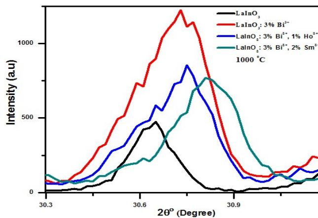
**Fig 1.** XRD patterns corresponding to (a) Pure LaInO<sub>3</sub> samples annealed at 700, 900 and 1000 °C samples (b) Comparison of shift in diffraction peak positions on doping. ( $2\theta^\circ$  from 30.68-30.82°).
