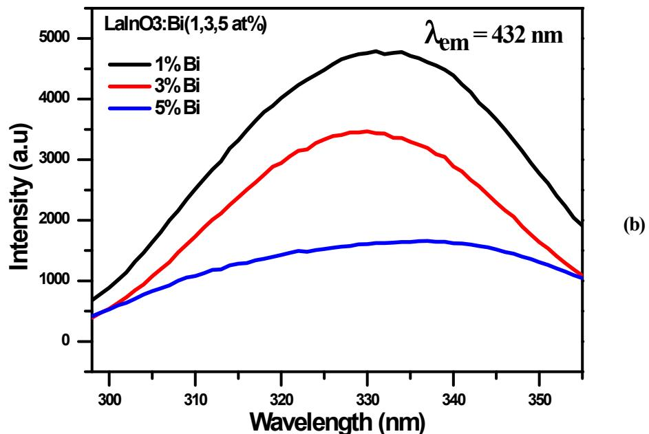
Fig. 3 Excitation spectra of LaInO<sub>3</sub>:Bi<sup>3+</sup> (1, 3, 5 at%) samples heat at 1000 °C
