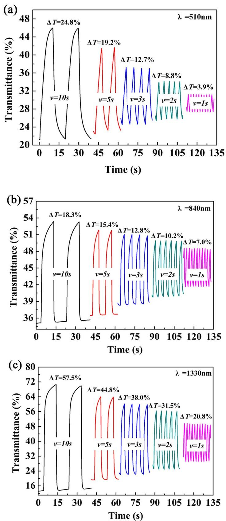
**Figure S5.** Electrochromic switching of P3 (a, b, c), with an interval of 10 s, 5 s, 3 s, 2 s, 1s.
