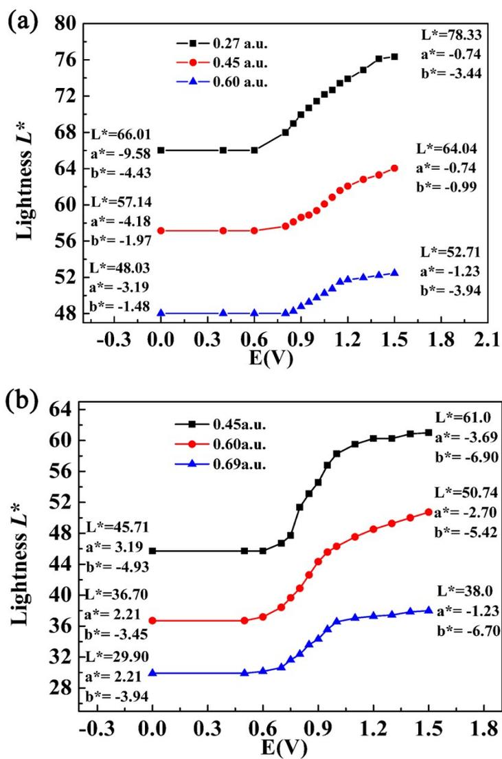
**Figure S6.** The  $L^* a^* b^*$  value of P1 (a), P3(b) with applied voltage from 0 V to 1.5 V.
