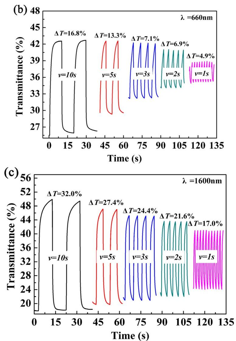
**Figure S4.** Electrochromic switching of P1(a, b, c), with an interval of 10 s, 5 s, 3 s, 2 s, 1s.
