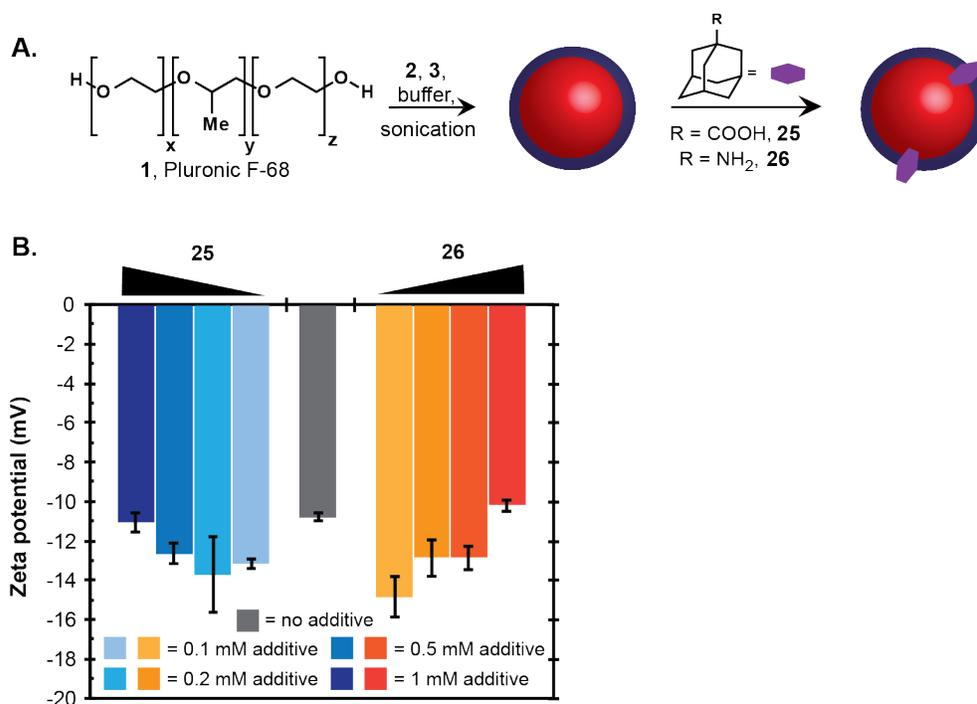
**Figure S3.** Pluronic-F68 control for the modification of perfluorocarbon emulsions using the adamantane- $\beta$ -cyclodextrin association. (A) Schematic for the control experiment. (B) Pluronic-F68 nanoemulsions were prepared and varying amounts of **25** or **26** in acetonitrile were added. The acetonitrile was removed by evaporation and the surface charge of the treated nanoemulsions was measured. Error bars represent the average of five zeta potential measurements.
