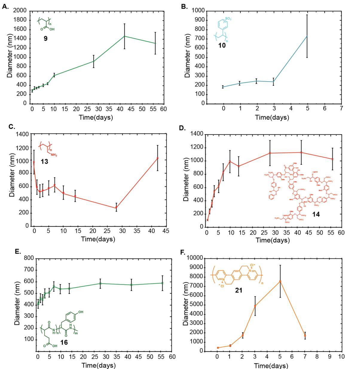
**Figure S1.** Stability of emulsions prepared from hydrophilic polymers. Emulsions were synthesized by dissolving the indicated polymer in PBS (2.8 wt%, except for **21** where solubility limited the polymer to 1.6 wt%) and sonicating in the presence of 7:3 PFD/PFTPA (20 wt%). Error bars represent the polydispersity as measured by DLS.
