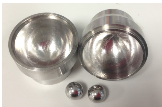
Figure S 12 46 mL large scale stainless steel snap closure grinding jars with two ½ inch ID hardened stainless steel ball bearings (each 8.22g).
