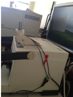
Figure S 9: Solenoid used as push-finger to automatically press the START button on the Retsch MM400
