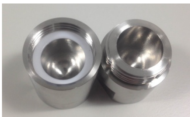
Figure S 11: 14.5mL Stainless steel screw closure grinding jars with Teflon washer
