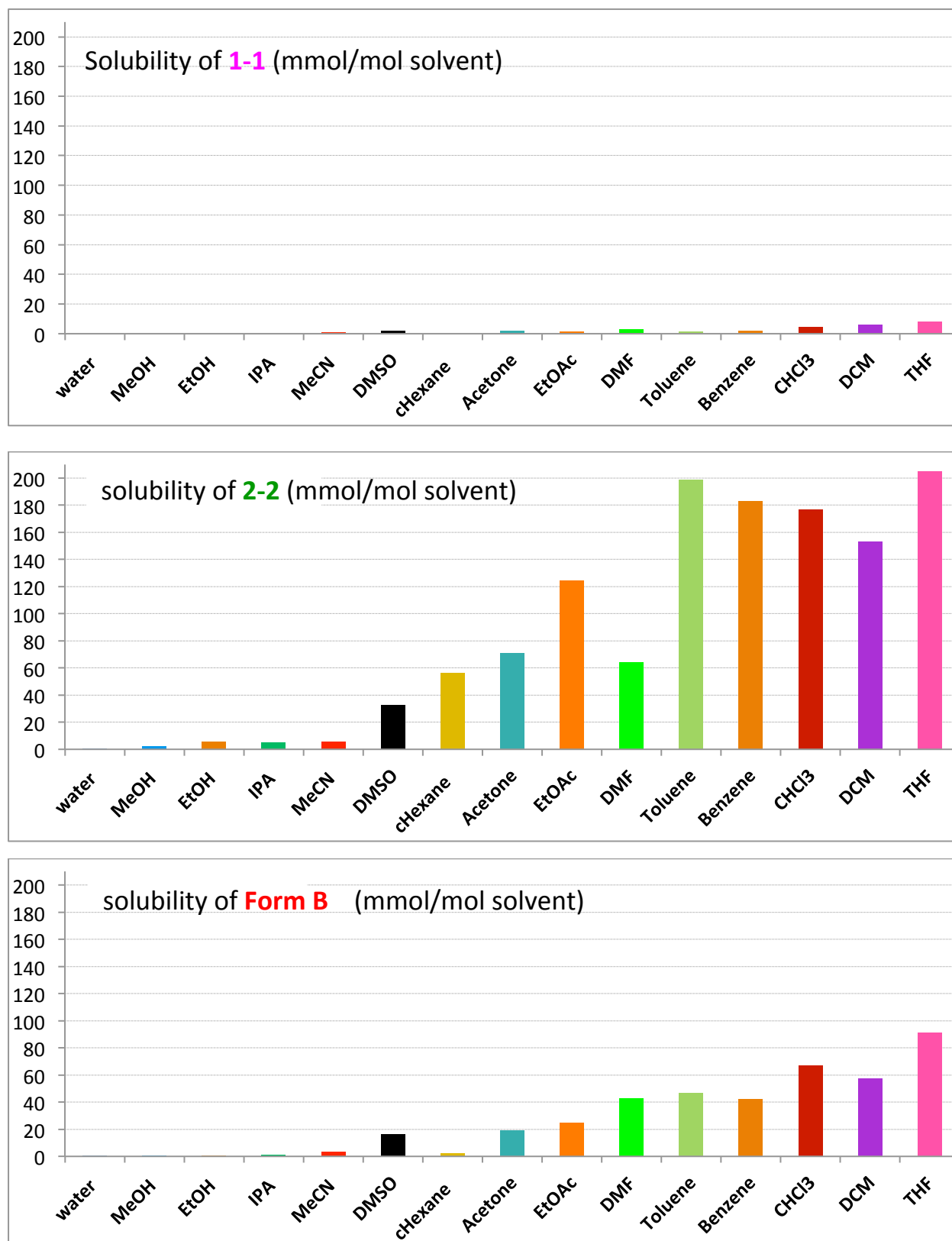
Figure S 84 Graphical representation of the solubility of 1-1, 2-2 and Form B in 15 solvents expressed as mmol/mol. As Form A transformed rapidly to Form B; the solubility of Form A is taken as that of Form B
