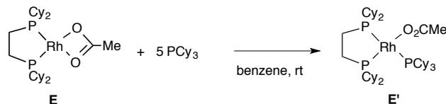
In a glovebox, to an NMR tube was added Rh(OAc)(dcype) **E** (5.8 mg, 0.01 mmol), PCy<sub>3</sub> (14.0 mg, 0.05 mmol) and benzene (0.5 mL) at room temperature and the mixture was stood for 1.5 h.
