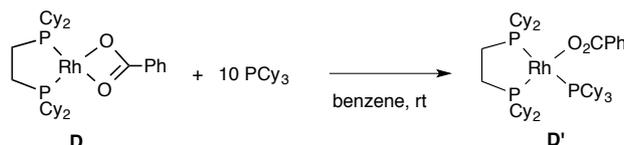
In a glovebox, to an NMR tube was added  $\text{Rh}(\text{O}_2\text{CPh})(\text{dcype})$  **D** (3.2 mg, 0.005 mmol),  $\text{PCy}_3$  (14.0 mg, 0.05 mmol) and benzene (0.5 mL) at room temperature and the mixture was stood for 1.5 h.
