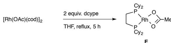
In a glovebox, a solution of 1,2-bis(dicyclohexylphosphino)ethane (1.69 g, 4.0 mmol) in THF (25 mL) was added dropwise to a solution of  $[\text{Rh}(\text{OAc})(\text{cod})]_2$  (1.08 g, 2.0 mmol) in THF (25 mL) and the mixture was refluxed for 5 h. The mixture was concentrated *in vacuo* and the residue was recrystallized from THF/pentane in a refrigerator to give **E** in 56 % yield (1.31 g, 2.24 mmol) as a yellow powder.<sup>iii</sup>
