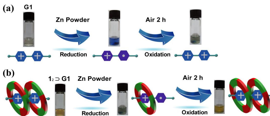
Figure S143 Graphical cartoon representation of redox control of (a) guest G1 and (b) complex 1_2 \supset G1 and photo showing color changes of redox-responsive complexation, solvent is argon-purged acetone.
