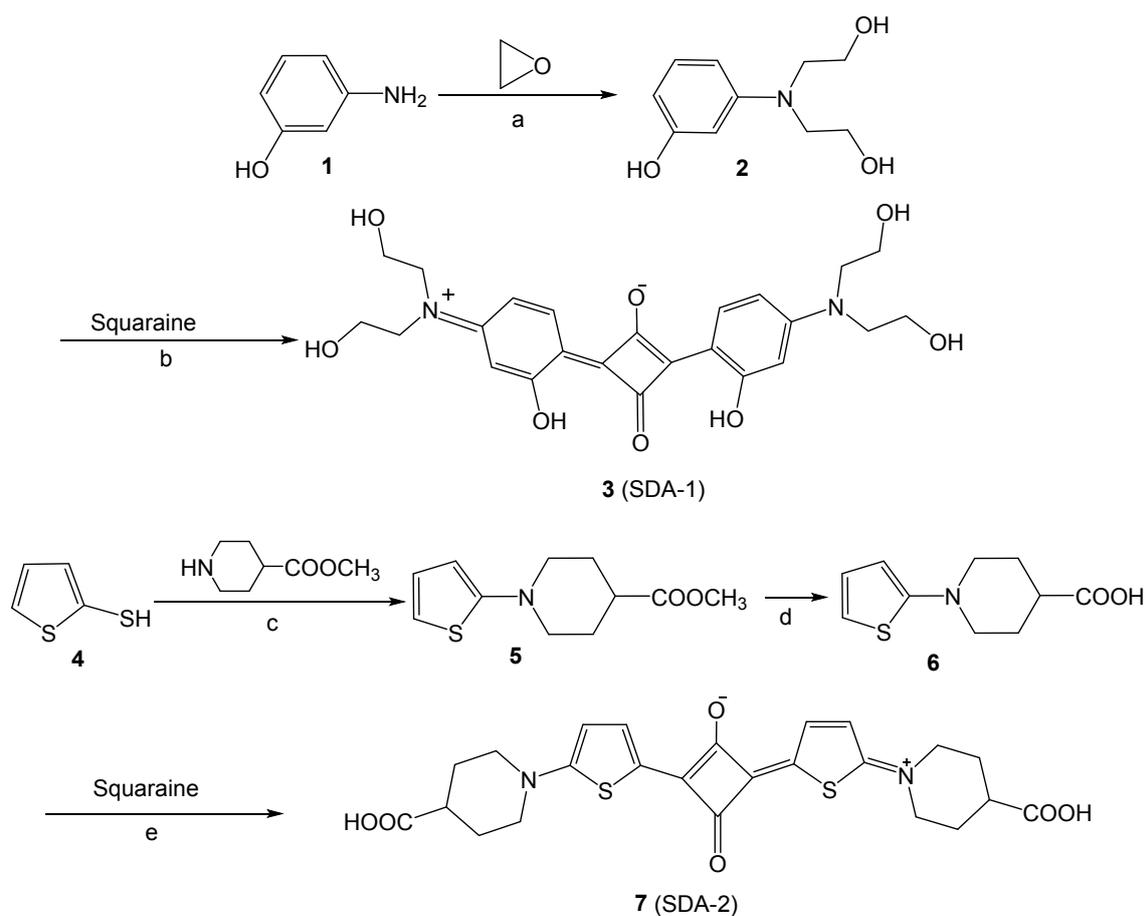
**Scheme S1<sup>a</sup>**. Synthetic routes of SDA-1, SDA-2. <sup>a</sup>Reagents and conditions: (a) Toluene, reflux, 1h; (b) (I) Toluene/1-butanol, reflux, 1 h; (II) NaHCO<sub>3</sub>, H<sub>2</sub>O; (c) THF, K<sub>2</sub>CO<sub>3</sub>; (d) (I) NaOH, H<sub>2</sub>O; (II) HOAc; (e) Toluene/1-butanol, reflux, 1 h.
