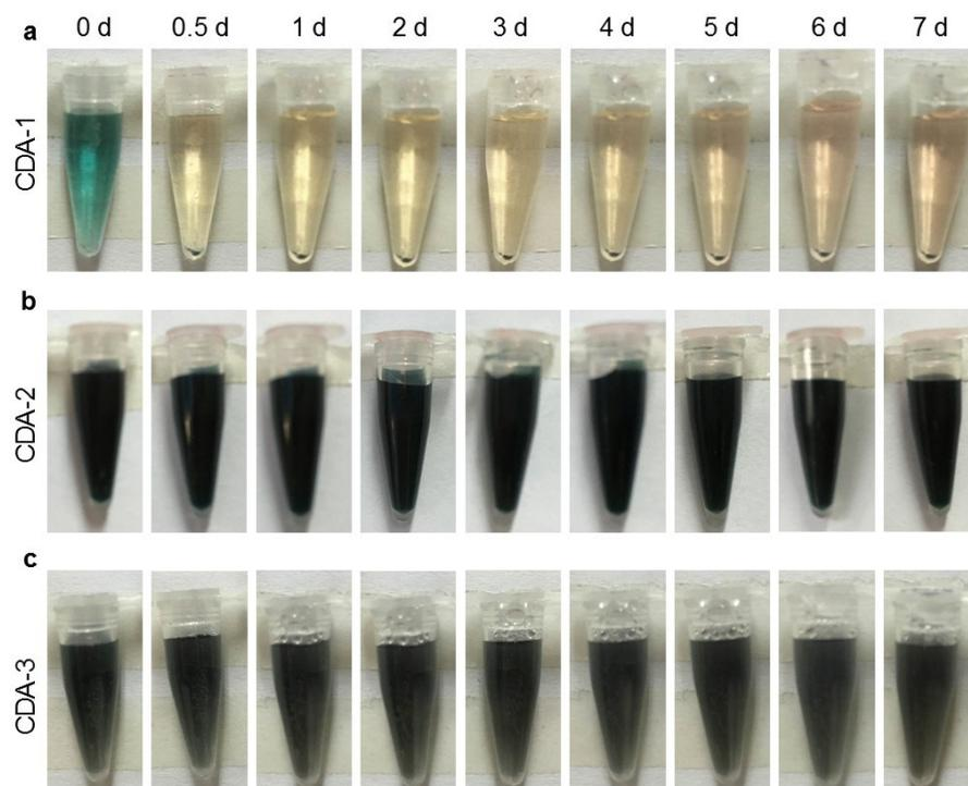
**Figure S11** The stability of CDA-1, CDA-2, and CDA-3 in water at room temperature after 7 day storage.
