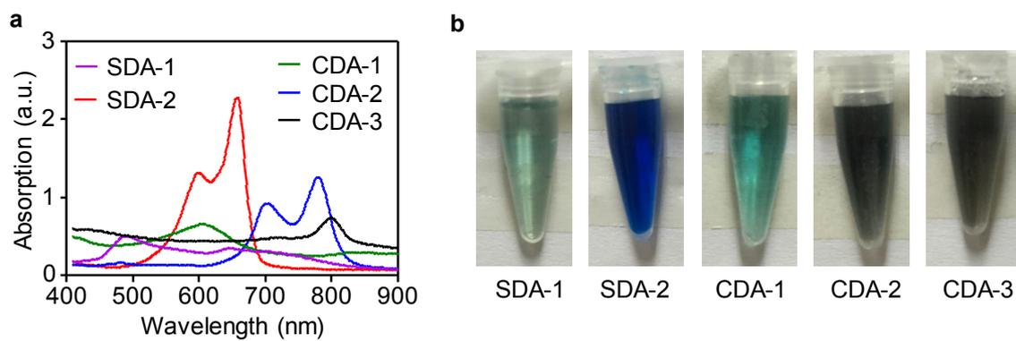
**Figure S10** (a) Absorption spectra recorded for SDA-1, SDA-2, CDA-1, CDA-2, and CDA-3 in water. (b) Corresponding photographs of SDA-1, SDA-2, CDA-1, CDA-2, and CDA-3.
