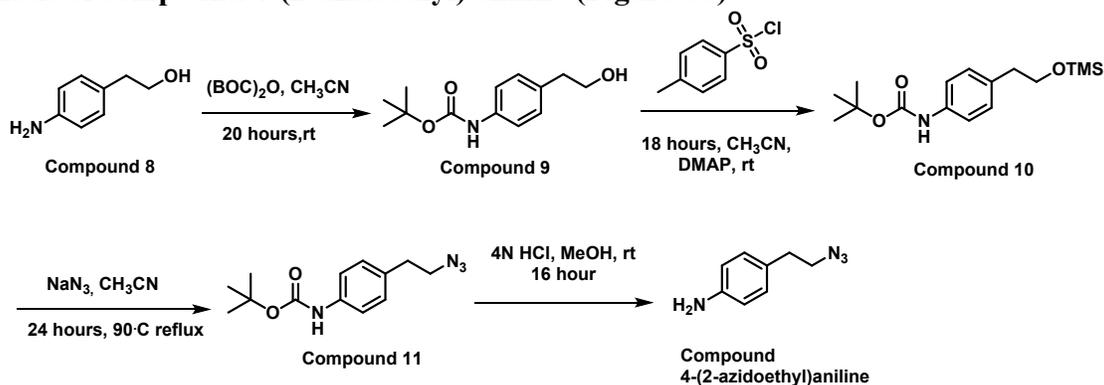
Figure S3. Synthesis of precursor compound 4-(2-azidoethyl) aniline.
