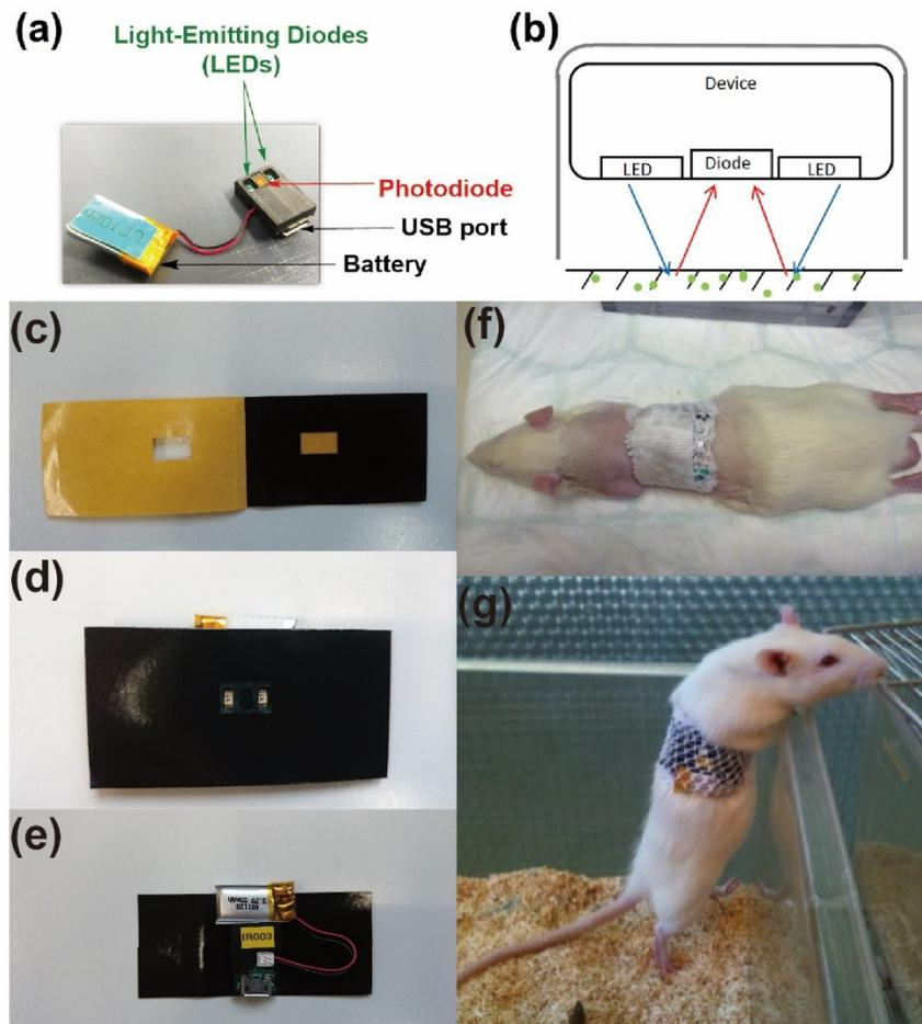
**Figure. S10.** (a) Transcutaneous device and battery used for the transcutaneous LED measurement, the photodiodes and LEDs in the device. (b) A schematic overview of the excitation and emission light between a transcutaneous device and fluorescent agents in capillary vessel after injection. (c-g) The fixation procedures of a transcutaneous device on the skin and measurements in a conscious rat.
