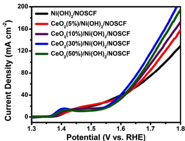
**Fig. S8** Polarization curves recorded on CeO<sub>2</sub>/Ni(OH)<sub>2</sub>/NOSCF electrode with different content of CeO<sub>2</sub> NPs in CeO<sub>2</sub>/Ni(OH)<sub>2</sub>/NOSCF. The loading mass ratio of CeO<sub>2</sub> NPs on Ni(OH)<sub>2</sub>/NOSCF were 5%, 10%, 30% and 50%, potential scan rate is 5 mV s<sup>-1</sup>.
