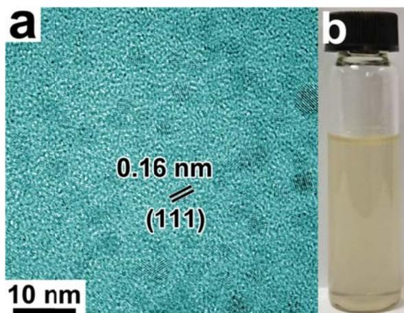
**Fig. S6** (a) TEM image of  $\text{CeO}_2$  NPs after surface modification. The interplanar spacing of 0.16 nm can be observed, which is corresponding to the (111) crystal plane of  $\text{CeO}_2$  NPs. (b) Digital photo for surface modified- $\text{CeO}_2$  NPs dispersed in water solution.
