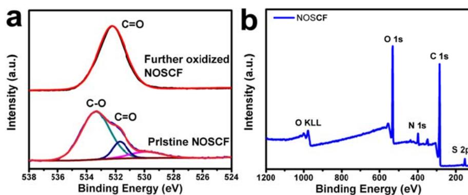
**Fig. S2** (a) High-resolution O 1s XPS spectra of NOSCF and further oxidized NOSCF. (b) XPS spectrum of N, O and S doped carbon foam (NOSCF), the contents of C, N, O and S elements in NOSCF were measured to be about 66.8, 4.3, 24.5 and 0.42 atom %, respectively.
