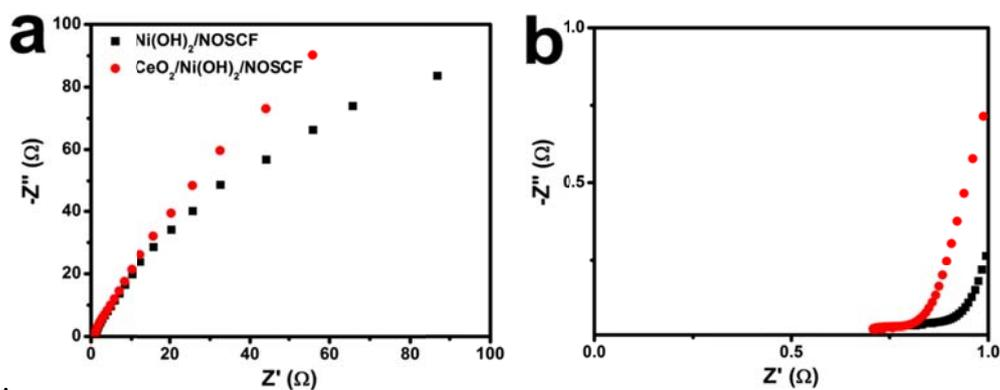
**Fig. S7** (a) EIS Nyquist plots showing the electrode kinetics of  $\text{Ni(OH)}_2/\text{NOSCF}$  and  $\text{CeO}_2/\text{Ni(OH)}_2/\text{NOSCF}$ . (b) Enlarged EIS Nyquist plots derived from a).
