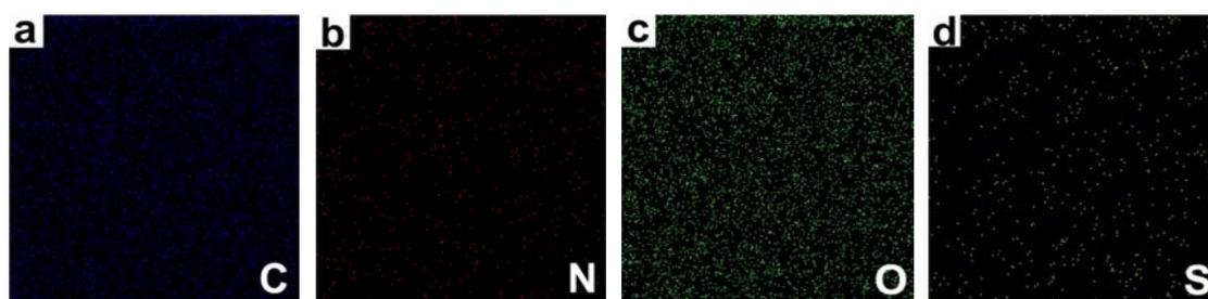
**Fig. S1** EDS elemental mapping for C, N, O and S elements recorded on the pure carbon foam.
