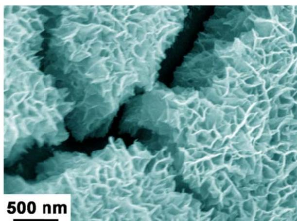
**Fig. S3** The enlarged SEM image of Ni(OH)<sub>2</sub> nanosheets grown on NOSCF.
