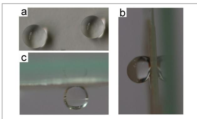
**Fig.S2** Images of water droplets of 4  $\mu\text{L}$  on the PLA-v surface with different tilt angles: (a) 0°, (b) 90°, and (c) 180°.
