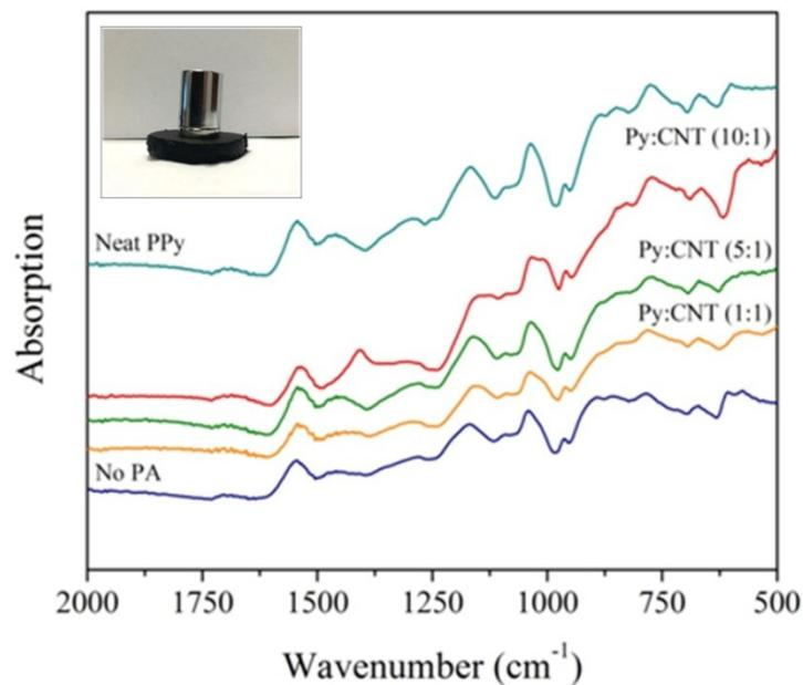
**Figure S6.** FTIR spectra of the neat PPy, PPy/CNT, and no PA hydrogels
