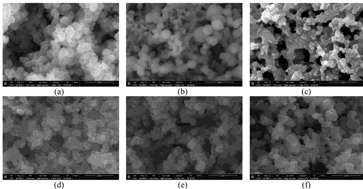
**Figure S4.** SEM micrographs of (a) No PA, (b) Neat PPy, (c) Py:CNT ratio of 10:1, (d) Py:CNT ratio of 5:1, (e) Py:CNT ratio of 2:1, and (f) Py:CNT ratio of 1:1
