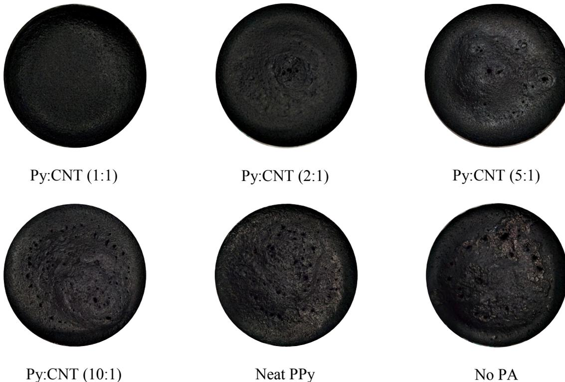
**Figure S1.** Surface of the resulting hydrogels after the tri-component reaction indicating the decrease in the amount of PPy produced by increasing the weight ratio of CNT in the third solution
