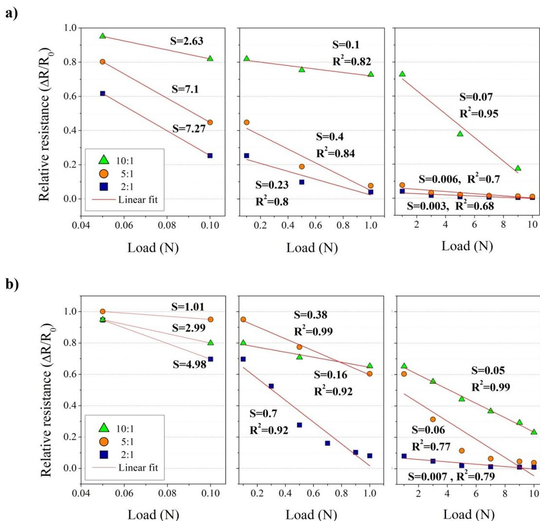
**Figure S8.** The relative resistance change and sensitivity of a) PPy/CNT, and b) PPy/GNP gels
