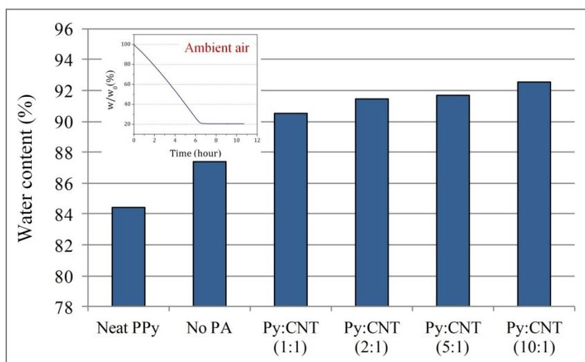
**Figure S2.** Water content of the neat PPy, No PA, and PPy/CNT samples dried in ambient air following by drying at 70°C. The graph on top left shows the drying time of a neat PPy sample in dried in ambient air.
