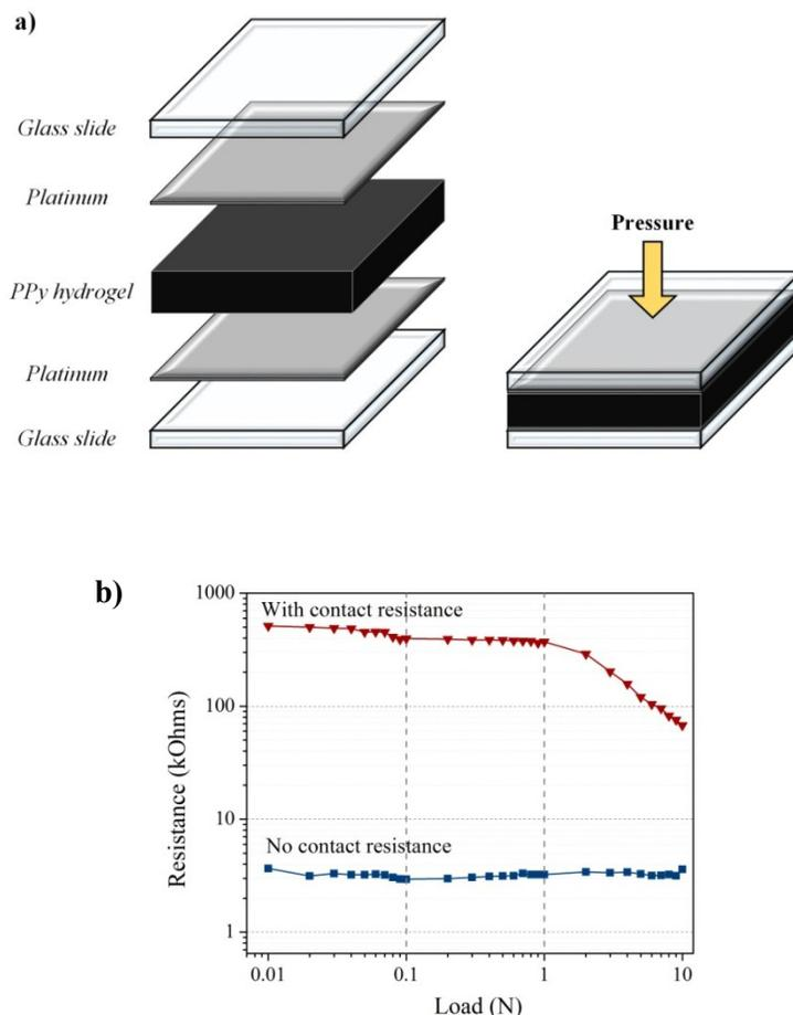
**Figure S7.** a) Schematic of the measurement setup to eliminate the contact resistance effect, and b) Piezoresistive response of a PPy/CNT hydrogel with and without the contact resistance effect
