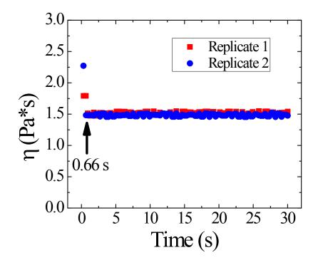
Figure S.3 Steady shear creep experiments performed at  $\sigma = 0.1$  Pa on a Newtonian viscosity standard (Cannon) following 300 seconds of oscillation at  $\sigma^* = 0.1$  Pa and  $\omega = 1$  rad/s. Two replicate experiments were performed to establish the lag time of the instrument.
