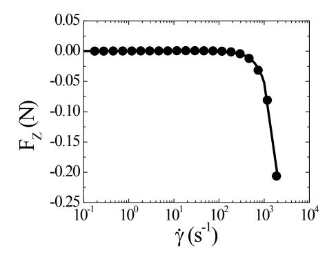
Figure S.1. Measured axial thrust as a function of the applied shear rate for a Newtonian PEG-200 solvent using a 40 mm  $2^0$  cone and plate tooling. The solid line is the expected contribution to the axial thrust from inertia given by Equation S.1.
