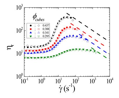
Figure S.2 Predicted elastohydrodynamic scaling (dashed lines) for the relative viscosity as a function of the shear rate for concentrated suspensions of cubic particles.
