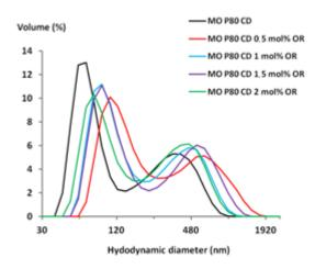
**Figure S7.** Determination of nano-object populations and hydrodynamic diameters [nm] through a multimodal model analysis of quasi-elastic light scattering data of self-assembled MO/5 mol% P80/OR nanocarriers produced upon dispersion of a mixed amphiphilic film encapsulating (a) 0 mol%; (b) 0.5 mol%; (c) 1 mol%; (d) 1.5 mol%, and (e) 2 mol% guest OR dye with respect to the lipid MO. Aqueous phase: Milli Q water. Temperature is 25°C.
