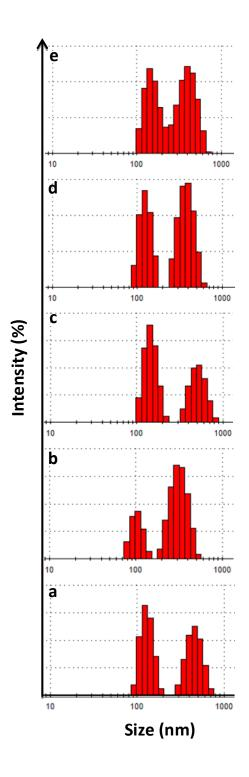
**Figure S8.** Determination of nano-object populations and hydrodynamic diameters [nm] through a multimodal model analysis of quasi-elastic light scattering data of self-assembled MO/5 mol% P80/β-CD-nC<sub>10</sub>/OR nanocarriers (4 mol% βCD-nC<sub>10</sub> deep cavitand content) produced upon dispersion of a mixed film encapsulating (a) 0 mol%; (b) 0.5 mol%; (c) 1 mol%; (d) 1.5 mol%, and (e) 2 mol% guest OR dye with respect to the lipid MO. Aqueous phase: Milli Q water. Temperature is 25°C.
