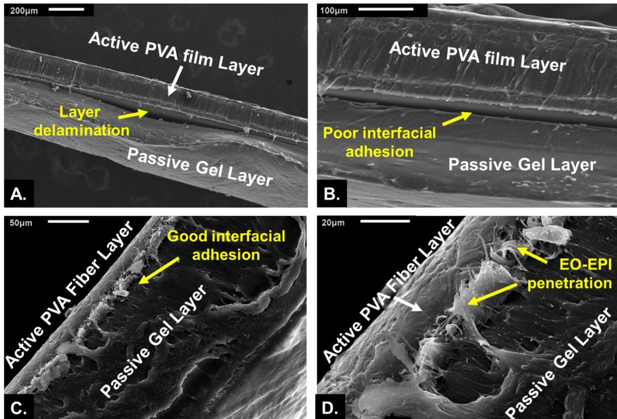
**Figure S2:** Cross-sections of bilayer composites containing either a PVA film or nanofiber mat
