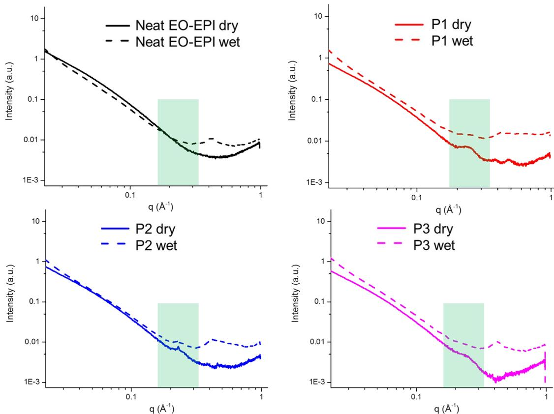
**Figure S5:** Small-angle X-ray Scattering (SAXS) of neat EO-EPI and wet and dry passive layer controls (P1- P3).
