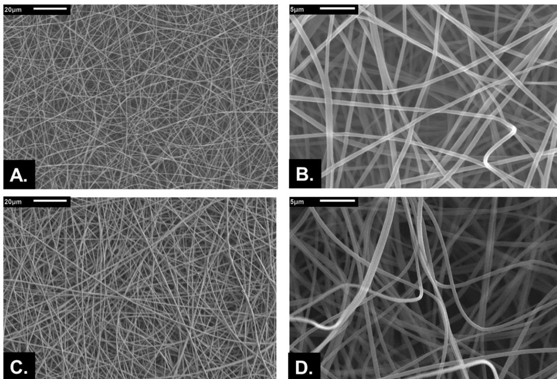
**Figure S1:** Scanning electron microscopy (SEM) of PVA nanofiber mats
