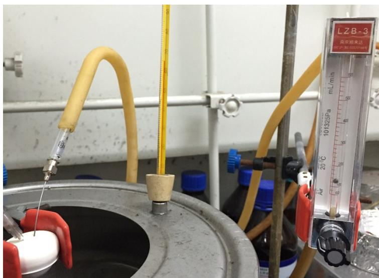
Fig. S3 The equipment for purging Ar into the suspensions at 65 °C and at the speed of 0.1 L/min.
